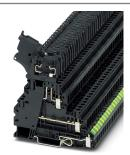
Fuse modular terminal block, fuse type: Glass / ceramics / ..., connection method: Screw connection, cross section:  $0.14 \text{ mm}^2$ -  $6 \text{ mm}^2$ , AWG: 26 - 10, nominal current: 28 A, nom. voltage: 500 V, width: 6.2 mm, fuse type:  $G / 5 \times 20$ , mounting type: NS 35/7.5, NS 35/15, color: black
