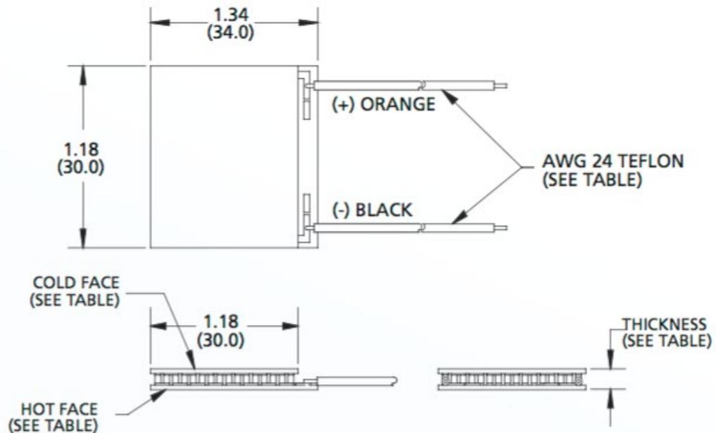
Ceramic Material: Alumina ( $Al_2O_3$ )
