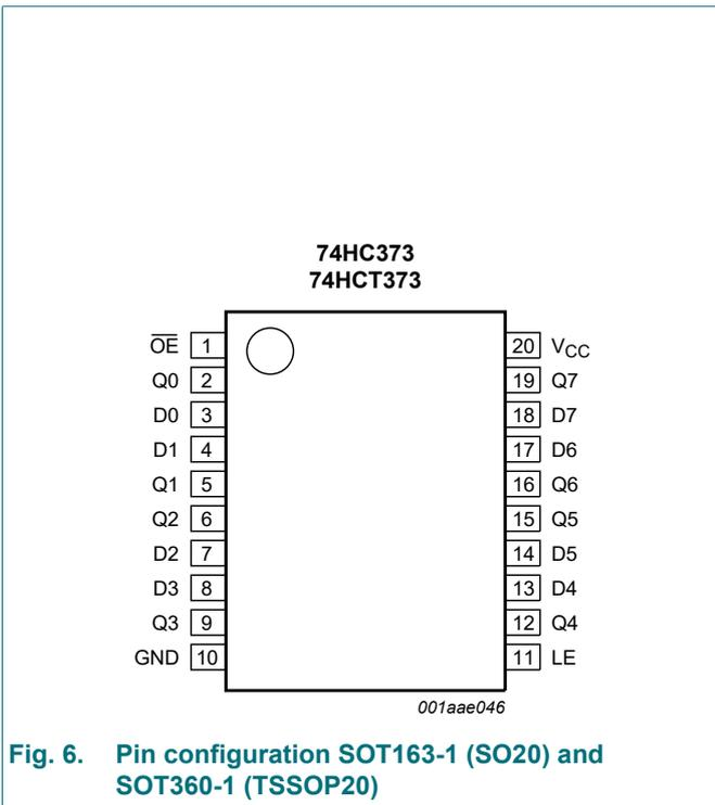
Fig. 6. Pin configuration SOT163-1 (SO20) and SOT360-1 (TSSOP20)
