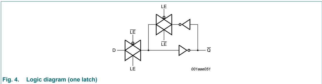
Fig. 4. Logic diagram (one latch)
