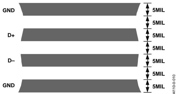
Figure 24. Typical Arrangement of Signal Tracks
