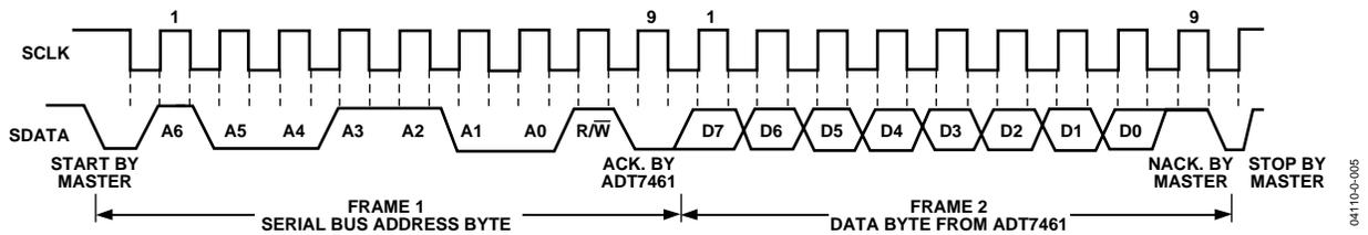
Figure 19. Reading from a Previously Selected Register
