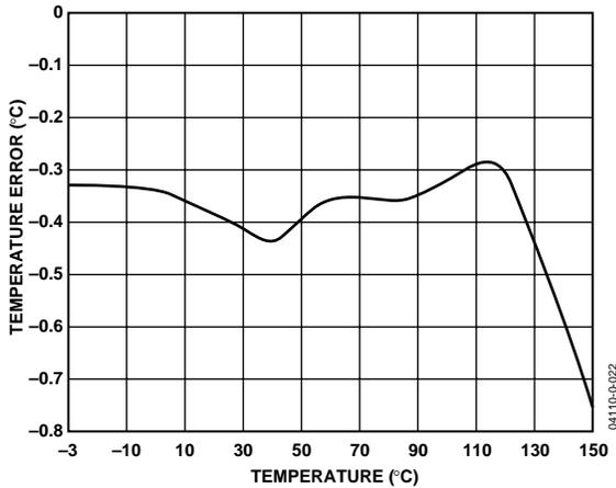
Figure 5. Temperature Error vs. Actual Temperature Using 2N3906
