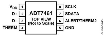
Figure 3. Pin Configuration
