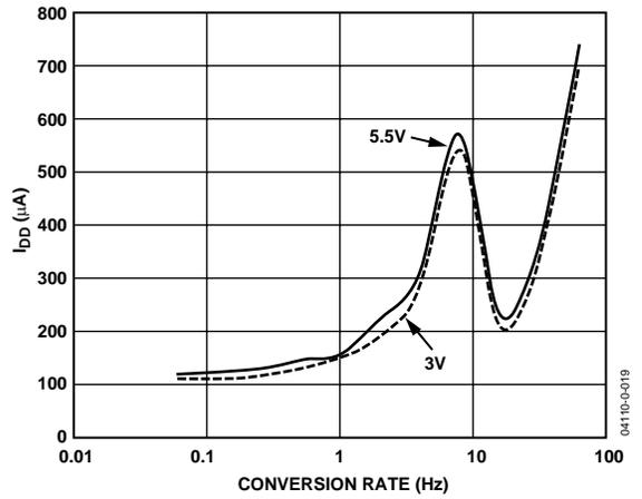
Figure 14. Operating Supply Current vs. Conversion Rate
