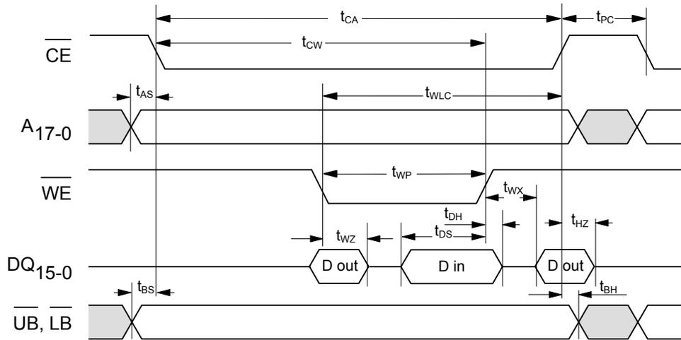
Figure 12. Write Cycle Timing 2 ( $\overline{CE}$  Controlled)
