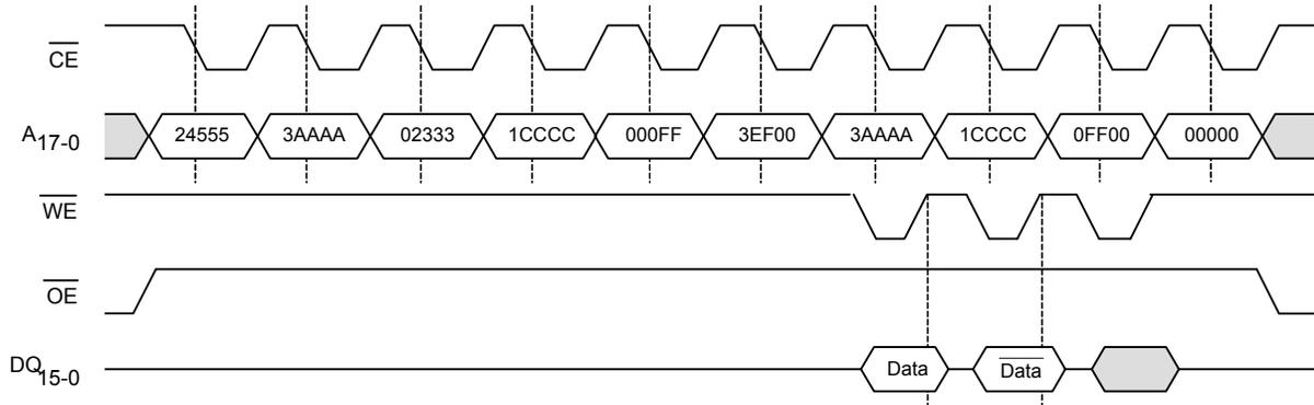
Figure 4. Sequence to Read Write-Protect Settings [1]
