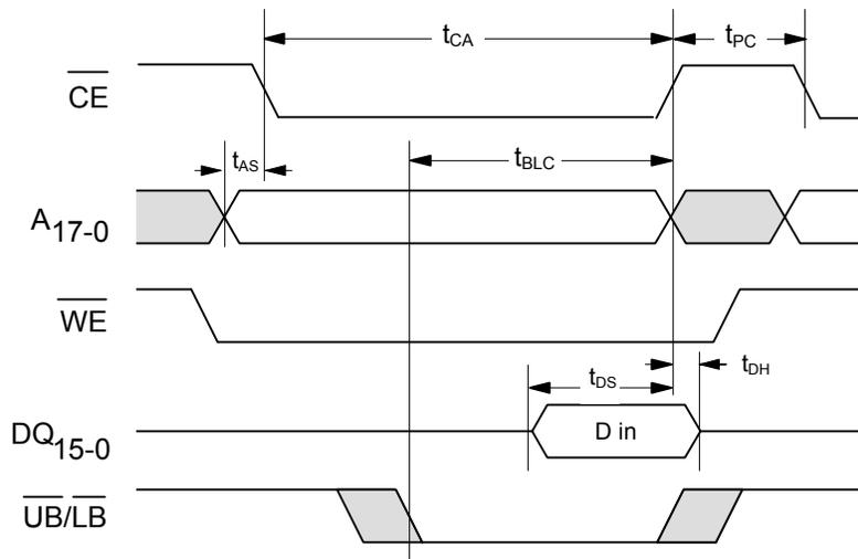
Figure 13. Write Cycle Timing 3 ( $\overline{CE}$  LOW) [10]
