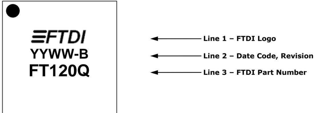
**Figure 9-4 QFN-28 Package Markings**
