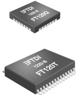
The FT120 is a USB controller developed independently with close consideration of the industry classic, D12 chip. It communicates with a microcontroller over the generic parallel interface. The FT120 has the following advanced features:
