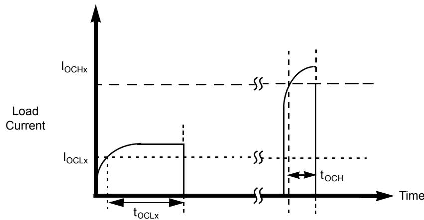
**Figure 5. Overcurrent Shutdown**
