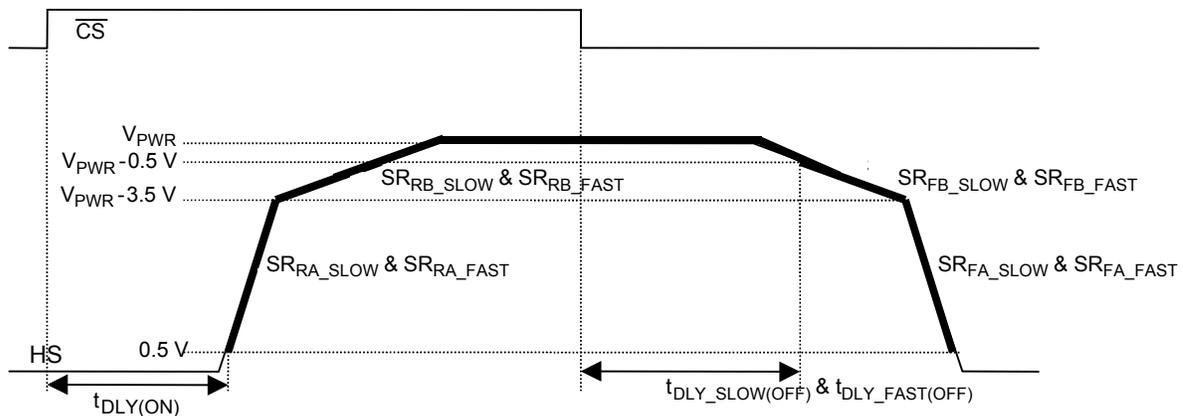
**Figure 4. Output Slew Rate and Time Delays**
