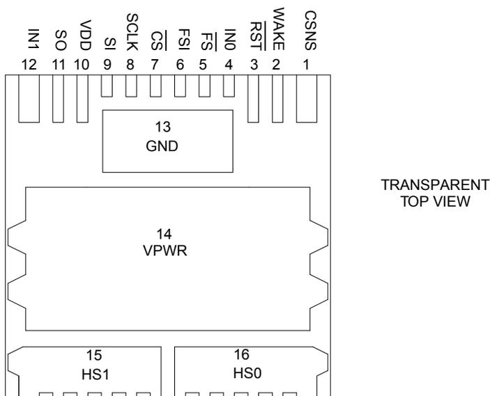
**Figure 3. 34984 Pin Connections (Transparent Top View)**
