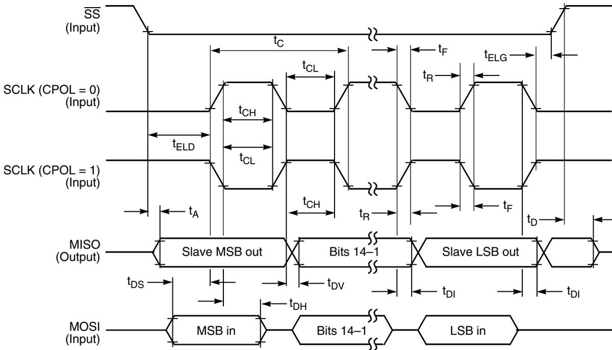
Figure 17. SPI Slave Timing (CPHA = 0)
