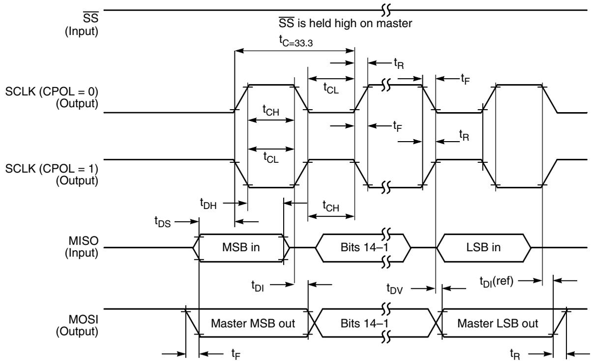
**Figure 15. SPI Master Timing (CPHA = 0)**
