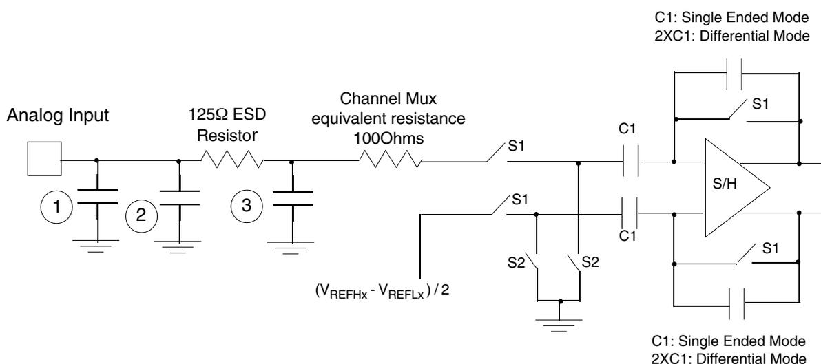
1. Parasitic capacitance due to package, pin-to-pin and pin-to-package base coupling; 1.8pF
