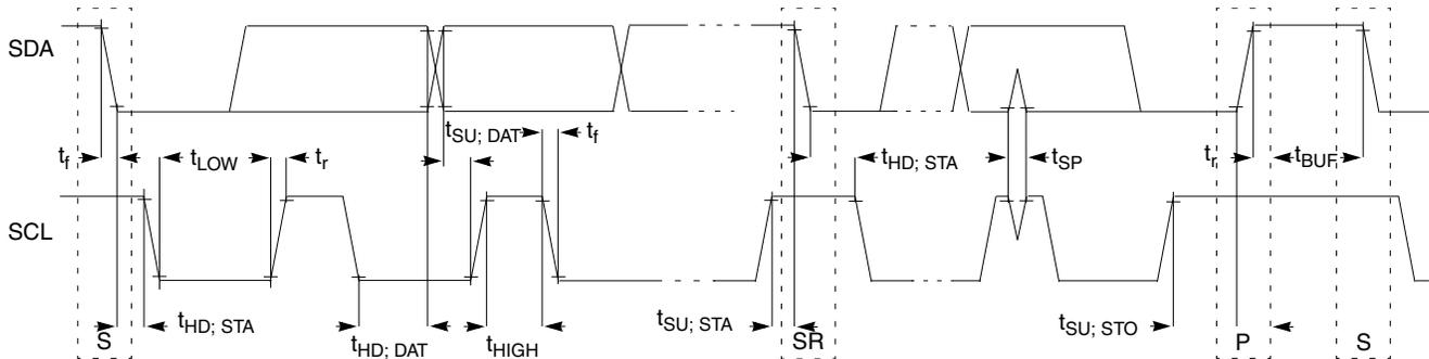
Figure 22. Timing Definition for Fast and Standard Mode Devices on the I<sup>2</sup>C Bus
