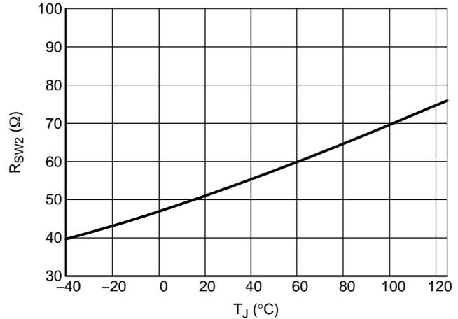
Figure 14. R<sub>SW</sub> at V<sub>CC</sub> = 15 V
