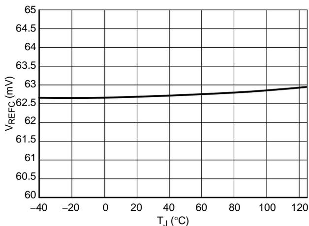
Figure 4.  $V_{REFC}$  at  $V_{CC} = 15$  V
