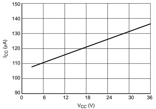
Figure 10.  $I_{CC}$  at  $T_J = 25^{\circ}C$  for NCP4328B
