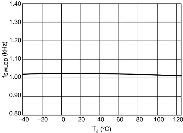
Figure 13. LED Switching Frequency at V<sub>CC</sub> = 15 V
