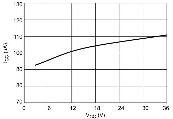
Figure 8.  $I_{CC}$  at  $T_J = 25^{\circ}C$  for NCP4328A
