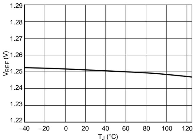
Figure 2.  $V_{REF}$  at  $V_{CC} = 15$  V
