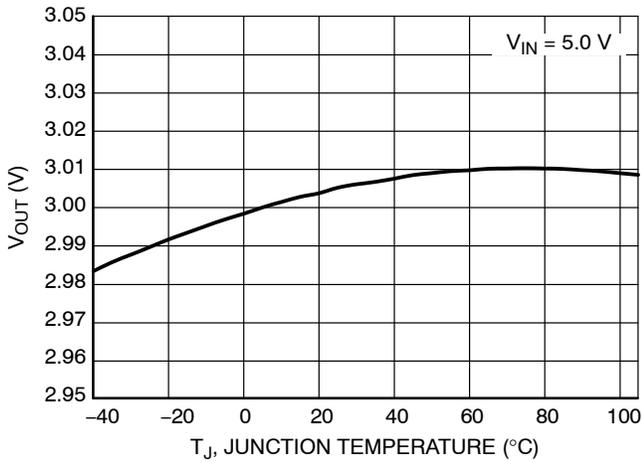
Figure 9. Output Voltage vs. Temperature, 3.0 V Version
