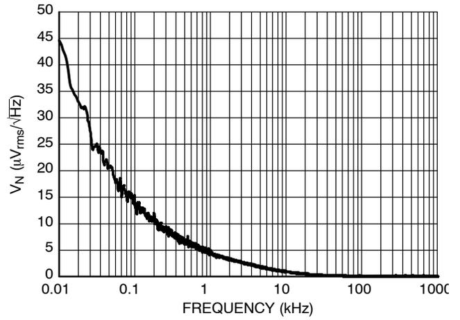
Figure 22. Output Voltage Noise, 8.0 V version,
