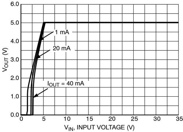
Figure 15. Output Voltage vs. Input Voltage, 5.0 V Version
