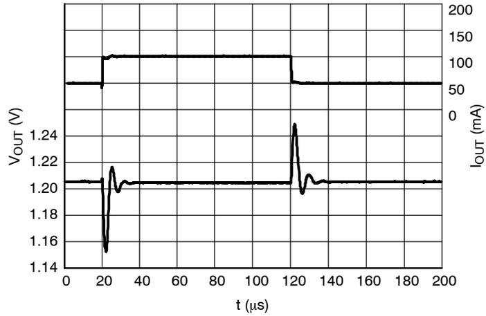
**Figure 26. Load Transients, 3.0 V Version,
