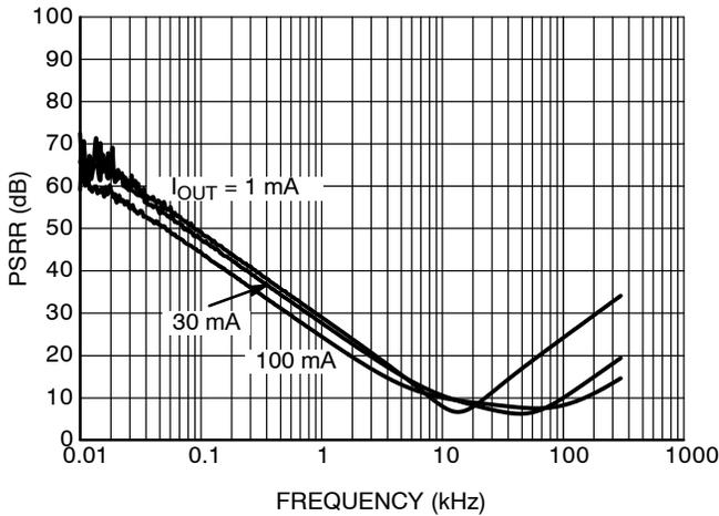
Figure 17. PSRR, 3.0 V Version,  $V_{IN} = 6.0$  V
