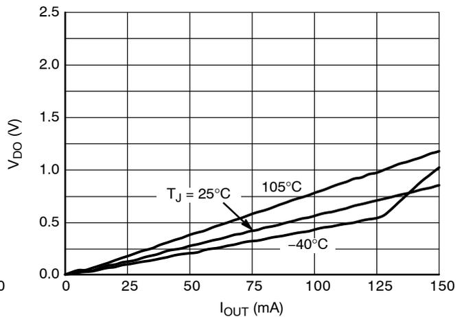
Figure 8. Dropout Voltage vs. Output Current
