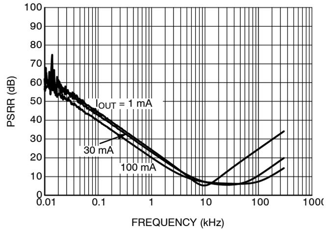
Figure 18. PSRR, 5.0 V Version,  $V_{IN} = 8.0$  V
