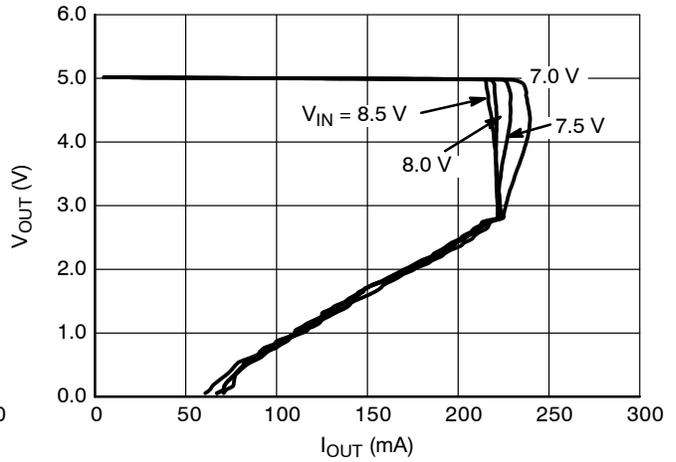
Figure 4. Output Voltage vs. Output Current
