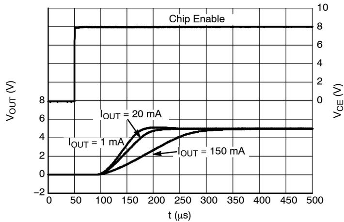
Figure 30. Start-up, 5.0 V Version,  $V_{IN} = 8.0 \text{ V}$
