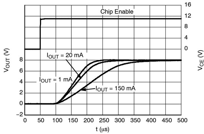
Figure 31. Start-up, 8.0 V Version,  $V_{\text{IN}} = 11.0 \text{ V}$
