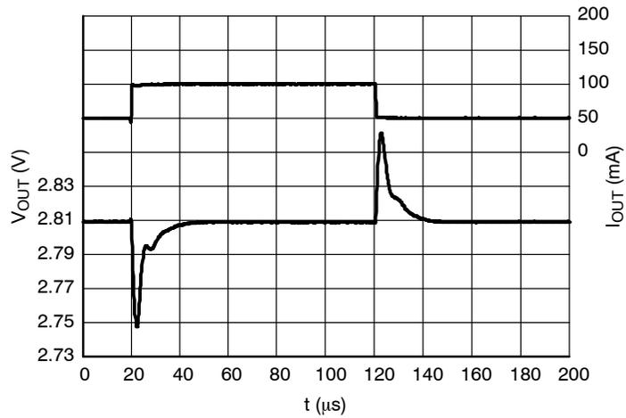
**Figure 27. Load Transients, 5.0 V Version,
