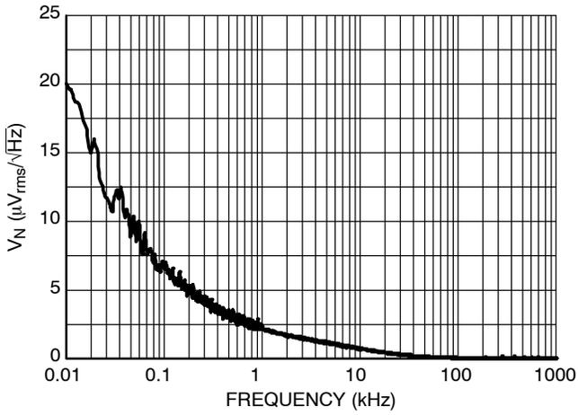
Figure 21. Output Voltage Noise, 5.0 V Version,
