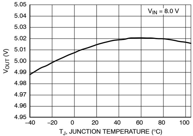
Figure 10. Output Voltage vs. Temperature, 5.0 V Version
