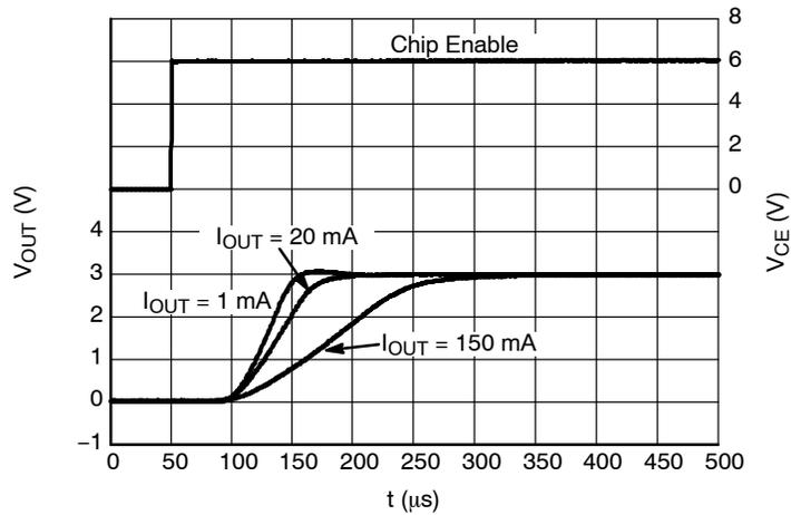
Figure 29. Start-up, 3.0 V Version,  $V_{IN} = 6.0 \text{ V}$
