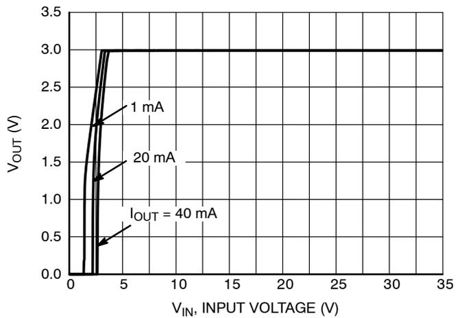
Figure 14. Output Voltage vs. Input Voltage, 3.0 V Version
