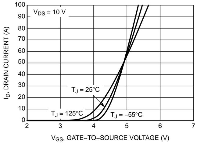
Figure 2. Transfer Characteristics
