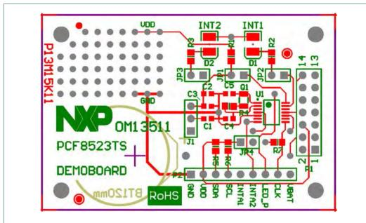
Fig 4. Demo board and top side layout
