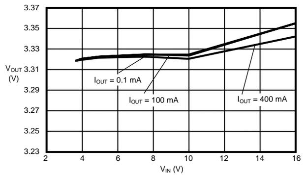
**(12) Output Voltage ( $V_{OUT}$ ) vs. Input Voltage ( $V_{IN}$ )
