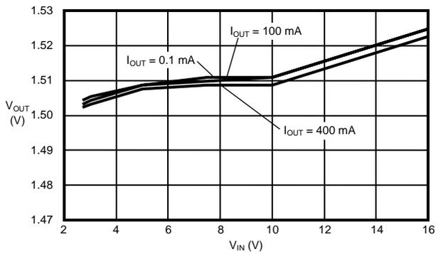
**(11) Output Voltage ( $V_{OUT}$ ) vs. Input Voltage ( $V_{IN}$ )
