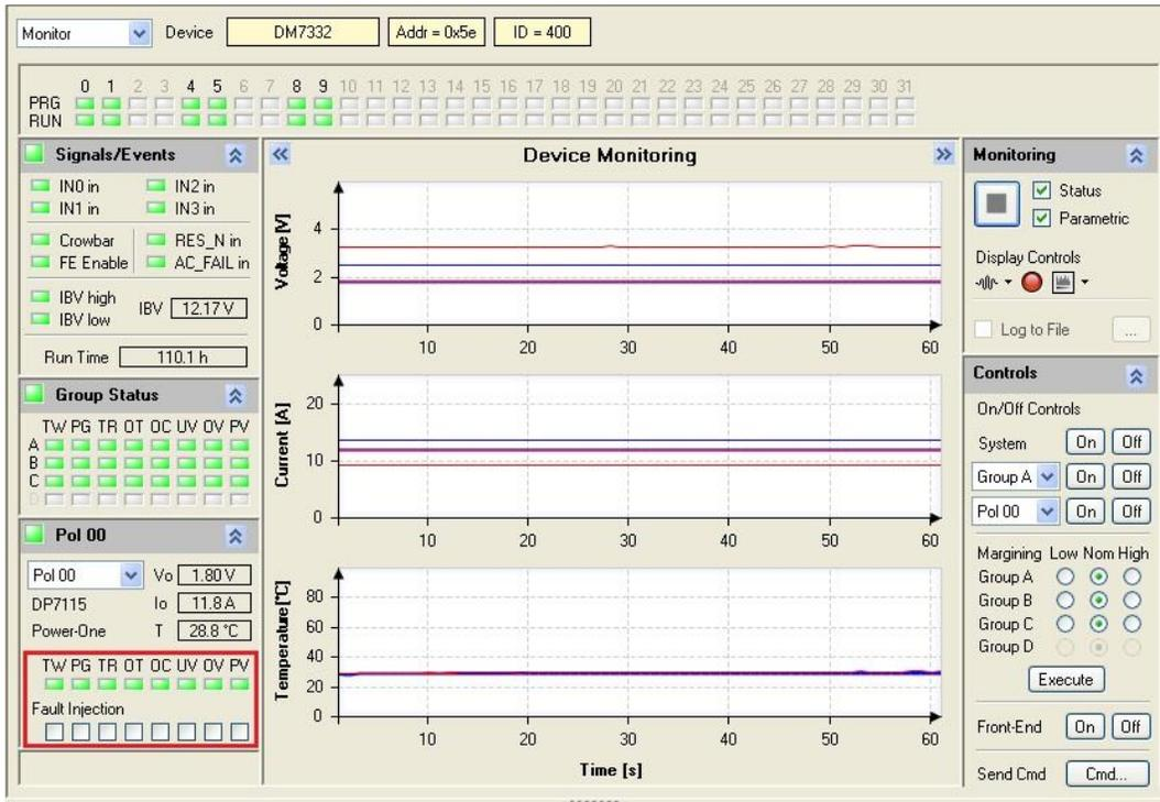
Fault injection into a dPOL requires selecting that dPOL in the POL status dialog in the left column of the Monitoring dialog window. As long as the checkbox is checked, the fault trigger is present in the dPOL. An injected fault is handled by the dPOL in the same fashion as an actual fault. It therefore gets propagated to the other dPOLs / Groups and shuts down in the programmed way the dPOL/Group/System as programmed for that fault.
