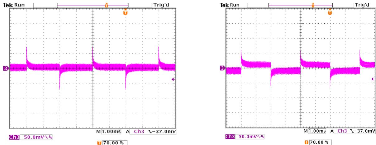
Figure 45. Transient Response with Regulation set to 0.55mV/A
