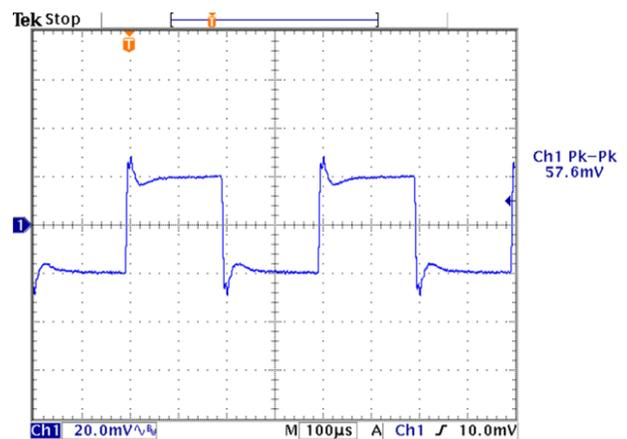
As the Load Regulation parameter is increased, step offsets in output voltage begin to appear, as shown in Figure 13. The Load Regulation parameter is an important part of Current Sharing. It is used to set one dPOL as a "master", by assigning a lower mV/A load regulation than all other dPOLs which share the load as "slaves". The dPOL with the lowest Regulation parameter sets the effective overall regulation. (See Current Sharing elsewhere in this document.)
