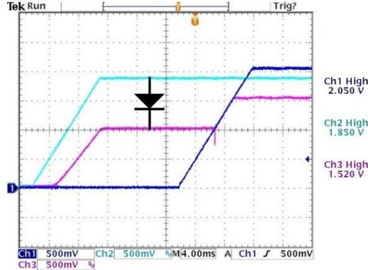
Figure 23 was captured with an actual system where a diode was added to pre-bias a 1.5V bus from a 1.85V bus in order to simulate the effect of current leakage through protection circuits of unpowered logic connected to powered logic outputs (a common source of pre-bias in power systems).
