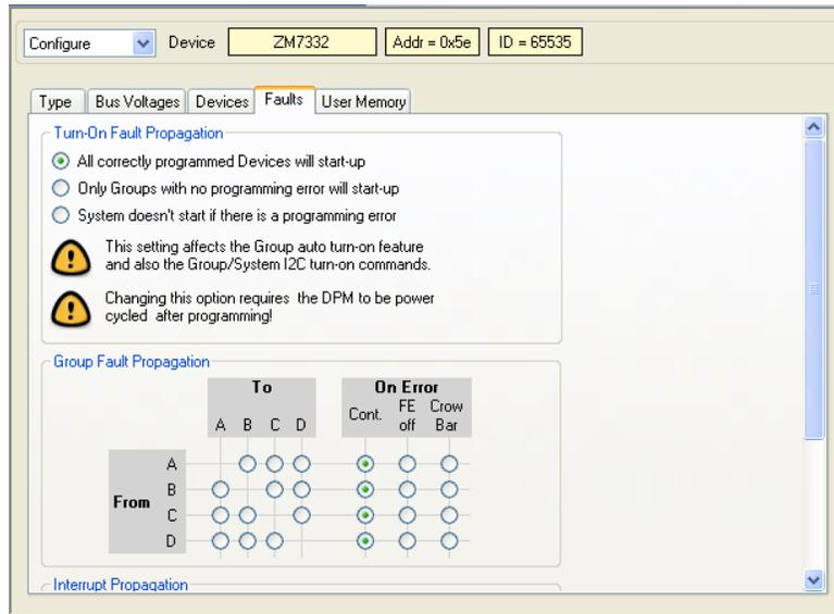
Note that the turn-off type of the fault as it propagates through the DPM will remain unchanged. Propagation options for dPOLs can be read or set in the dPOL PC3 register shown in Figure 33. The turn-off type of the fault propagation through the DPM will remain unchanged.
