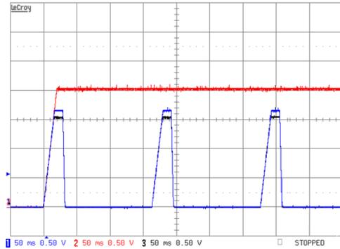
Since both Vo1 and Vo2 have the same delay and slew rate settings they will continue to turn off and on synchronously every 130ms as shown in Figure 37 until the condition causing the undervoltage is removed.
