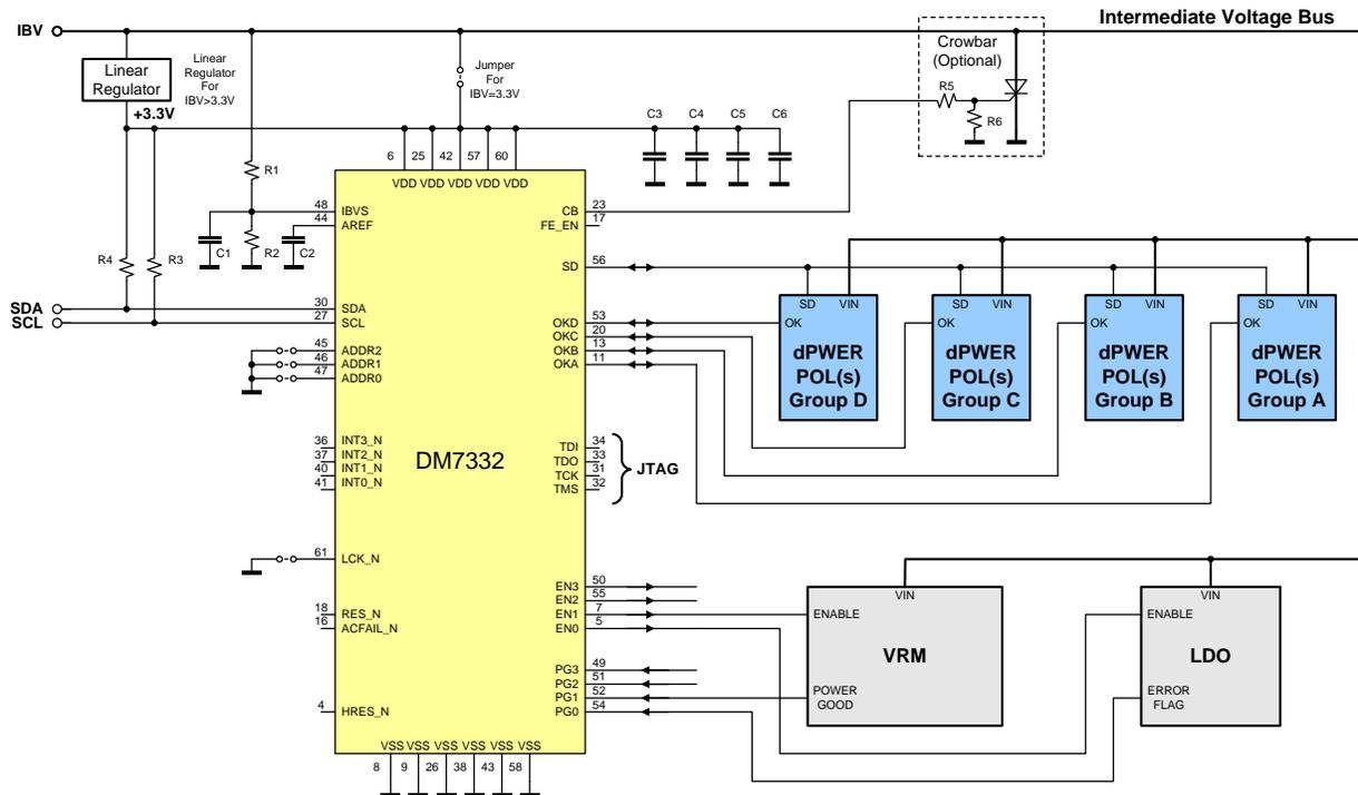
Shown in Figure 53 is a more detailed schematic of a typical application using a DM7300 series Digital Power Manager (DPM) and at least one DP8140G point-of-load converter (dPOL). Additional d-pwer® series dPOLs may be connected (Note SD and OK dashed lines "TO OTHER dPOLs"). As noted earlier, OK connections are determined by which group a given dPOL is assigned to in the user's application.
