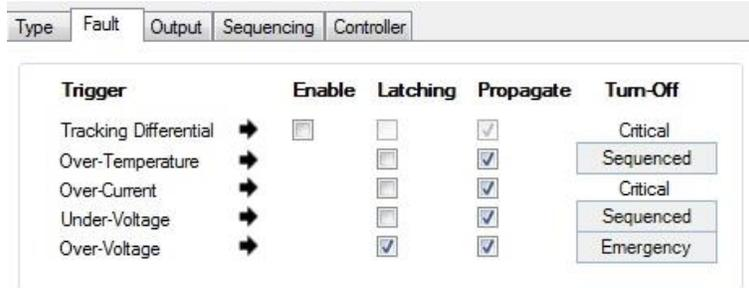
If the non-latching protection is selected, a dPOL will attempt to restart every 130ms until the condition that triggered the protection is removed. When restarting, the output voltages follow tracking and sequencing settings.
