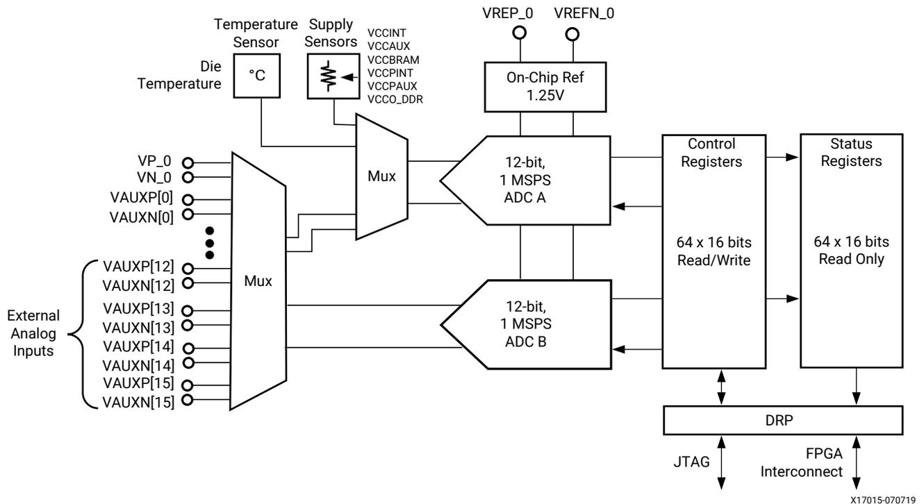
It is not necessary to instantiate the XADC in a design to access the on-chip monitoring capability. However, if the XADC is not instantiated in a design, the only way to access this information is through the JTAG test access port (TAP). To allow access to the status registers (measurement results) from the FPGA logic, the XADC must be instantiated.
