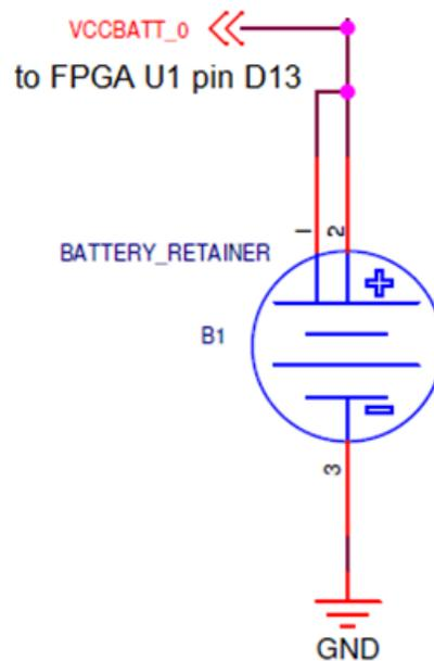
The Keystone 2998 battery retainer B1 is soldered to the board with the positive output connected to the FPGA U1 VCC\_PSBATT pin D13. The B1 retainer accepts a 6.8 mm 1.5V single-cell, coin type battery similar to Seiko part number SR621SW, silver oxide, 1.55V non-rechargeable battery.
