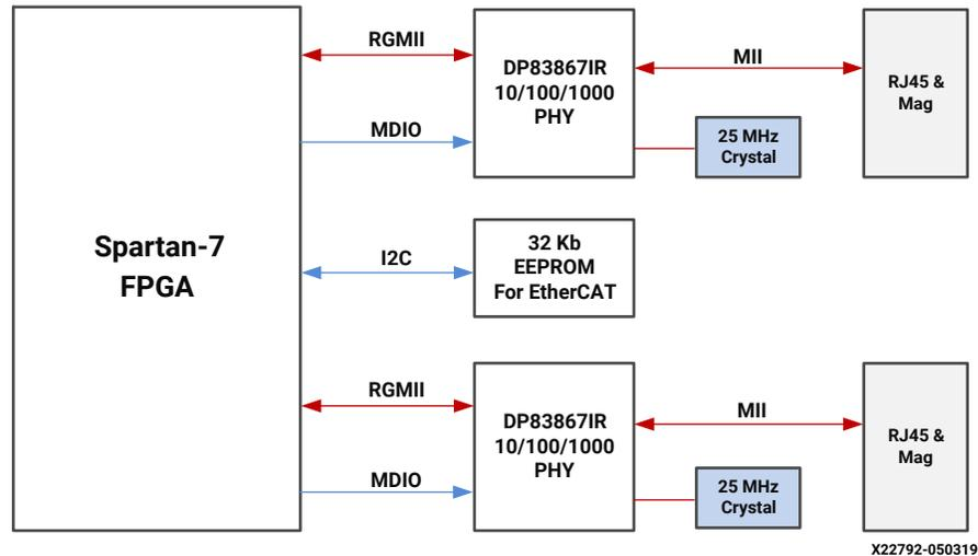
The SP701 evaluation board uses dual TI PHY device DP83867IRPAP (U14, U16) for Ethernet communications at 10 Mb/s, 100 Mb/s, or 1000 Mb/s. The board only supports the RGMII mode. Each PHY connects to a user-provided Ethernet cable through RJ-45 connector (J9, J11), Würth 7499111221A with built-in magnetics, and status LEDs. On power-up, or on reset, the PHY are configured to operate in the RGMII mode with the PHY addresses set by hardware strap settings:
