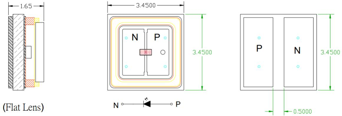
**Figure 2. IN-C35PUDDTU1 Package Dimension**
