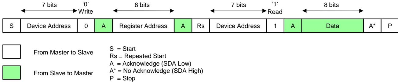
**Figure 7. I<sup>2</sup>C Read Cycle**
