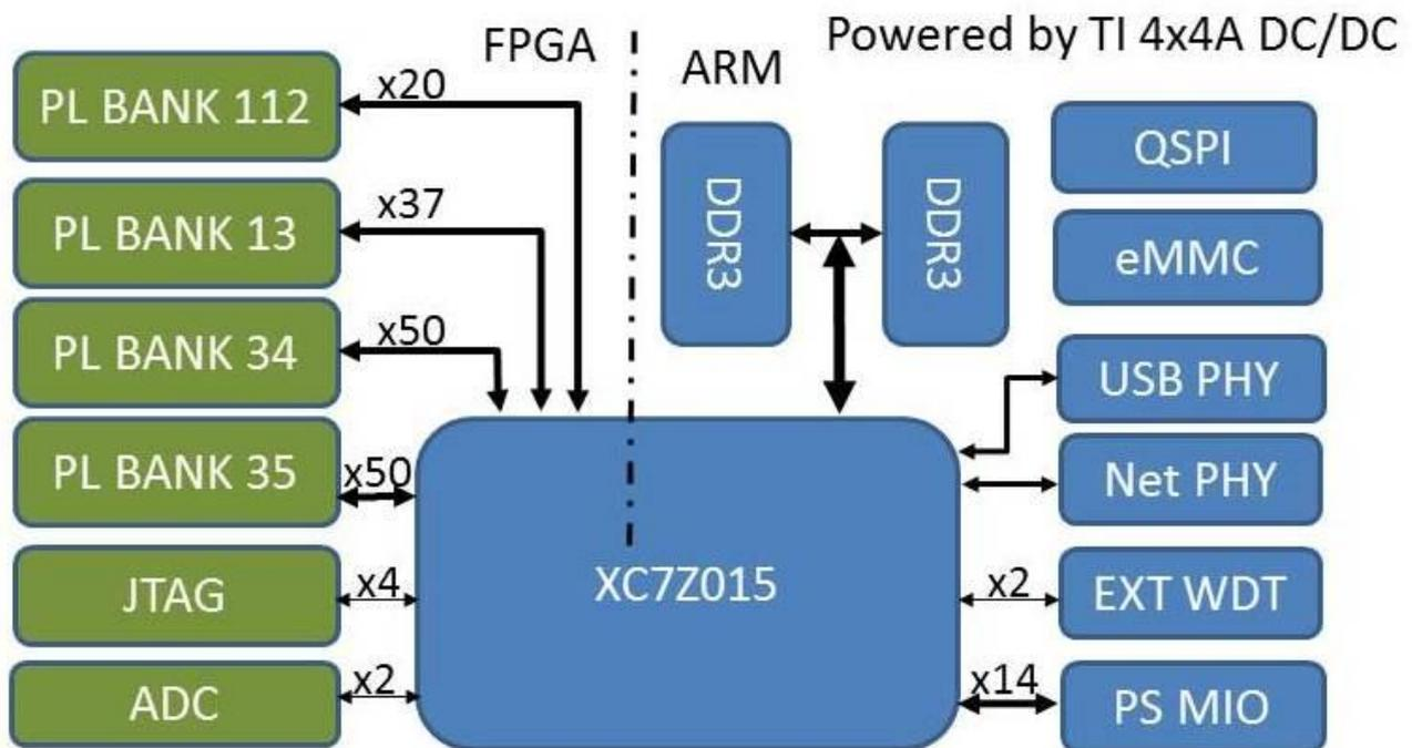
Figure 1-5 MYC-C7Z015 Function Block Diagram
