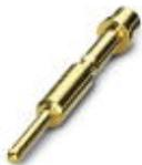
Crimp contact, turned, Single contact, Contact diameter: 1 mm, Crimp range: 0.14 mm<sup>2</sup>...0.5 mm<sup>2</sup>
