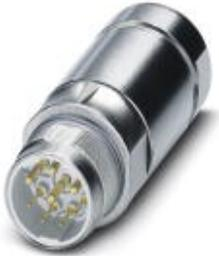
Coupler connector, straight long, Screw locking, M23, Number of positions: 4+3+PE, Type of contact: Male connector, Crimp connection, Shielded: Yes, Cable cross section: 9 mm...12 mm
