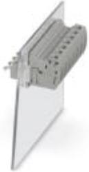
Panel feed-through terminal block, Connection method: Screw connection, Solder connection, Load current : 41 A, Cross section: 0.2 mm<sup>2</sup> - 6 mm<sup>2</sup>, Width: 8.1 mm, Color: gray
