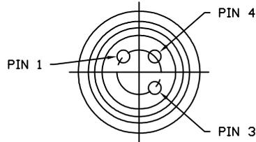
WHEN MATING WITH NORCOMP CONNECTORS, ONLY AN IP66 RATING CAN BE ACHIEVED IN MATING AREA BETWEEN CONNECTORS. CONNECTOR IS OTHERWISE IP67 AND MAY BE FULLY IP67 IF MATED WITH COMPETITOR PARTS.
