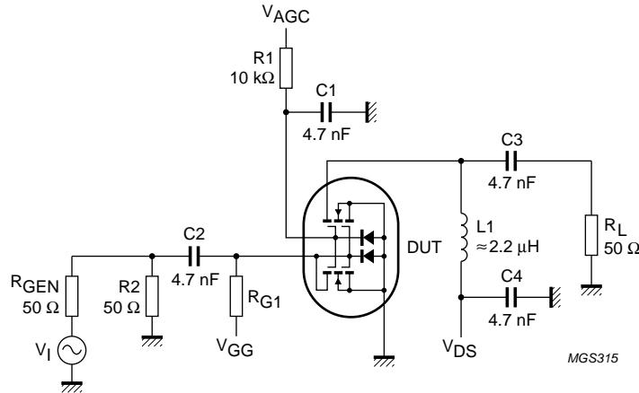
Fig.19 Cross-modulation test set-up (for one MOS-FET).
