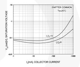
Figure 4. Collector-Emitter Saturation Voltage
