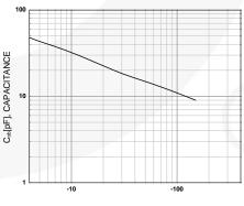
$V_{CB}[V]$ , COLLECTOR-BASE VOLTAGE
