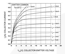
Figure 1. Static Characteristic
