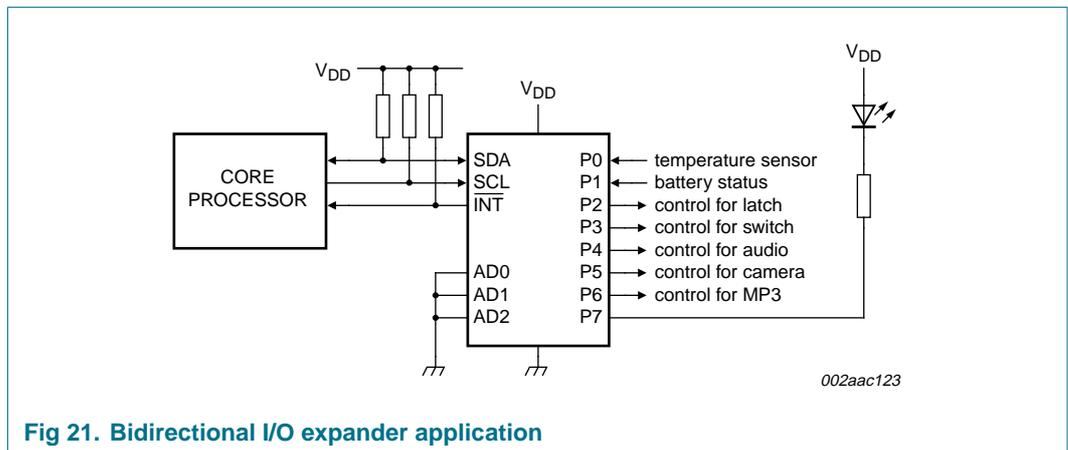
Fig 21. Bidirectional I/O expander application
