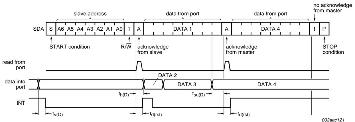
A LOW-to-HIGH transition of SDA while SCL is HIGH is defined as the STOP condition (P). Transfer of data can be stopped at any moment by a STOP condition. When this occurs, data present at the last acknowledge phase is valid (Output mode). Input data is lost.
