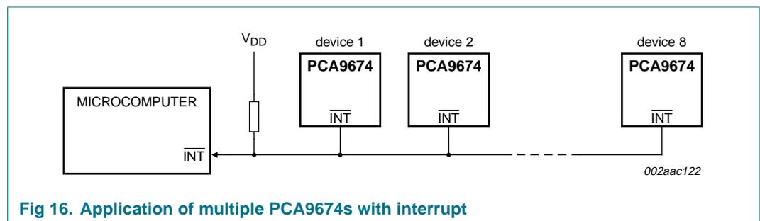
Fig 16. Application of multiple PCA9674s with interrupt
