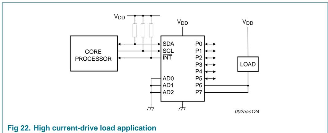
Fig 22. High current-drive load application
