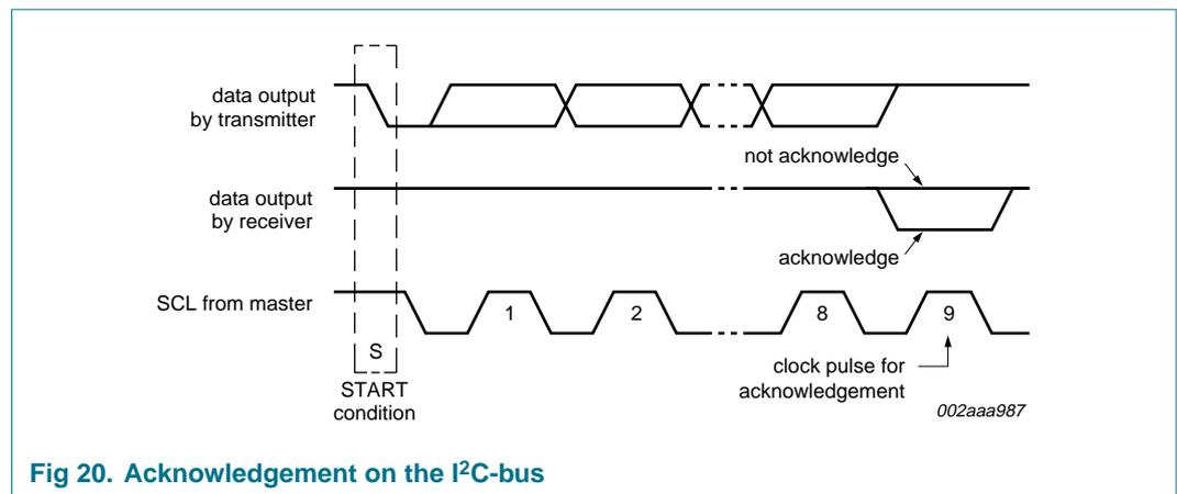
Fig 20. Acknowledgement on the I<sup>2</sup>C-bus
