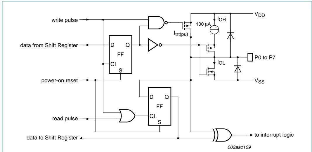
Fig 2. Simplified schematic diagram of P0 to P7
