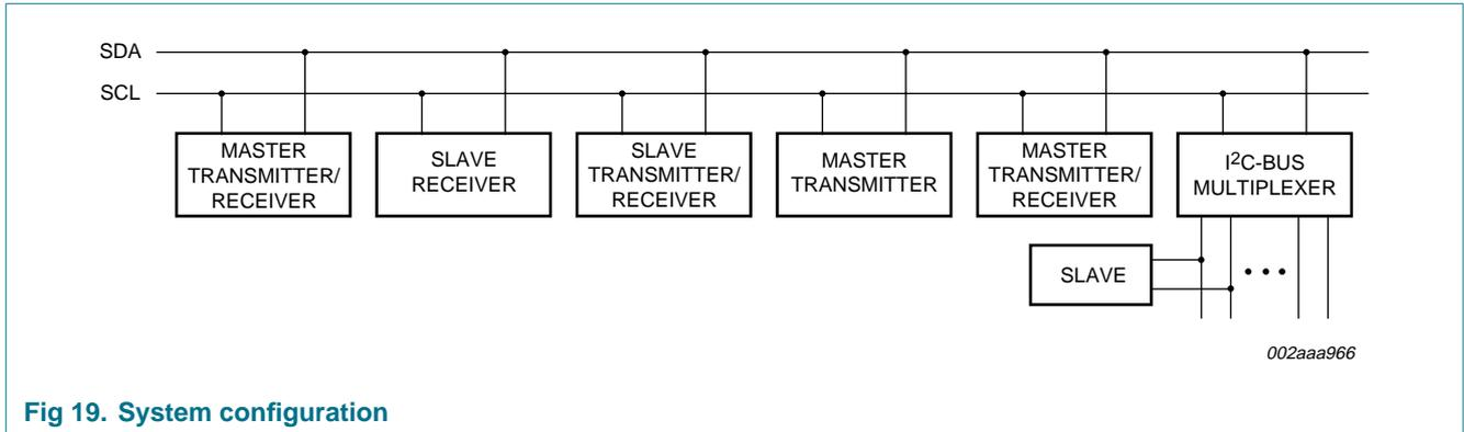
Fig 19. System configuration
