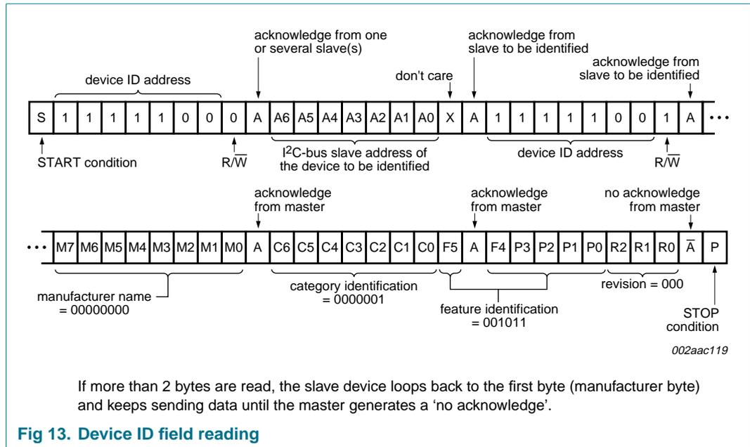
Fig 13. Device ID field reading
