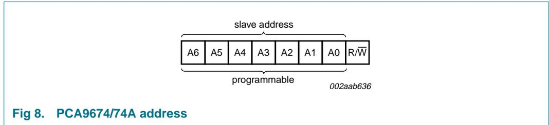
The last bit of the first byte defines the operation to be performed. When set to logic 1 a read is selected, while a logic 0 selects a write operation.
