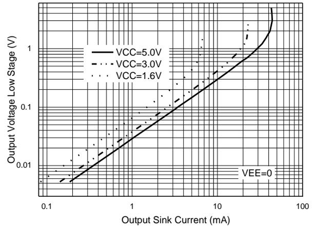
**Figure 10. Output Voltage vs. Output Sink Current**
