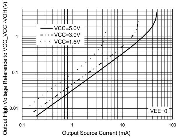
**Figure 9. Output Voltage vs. Output Source Current**
