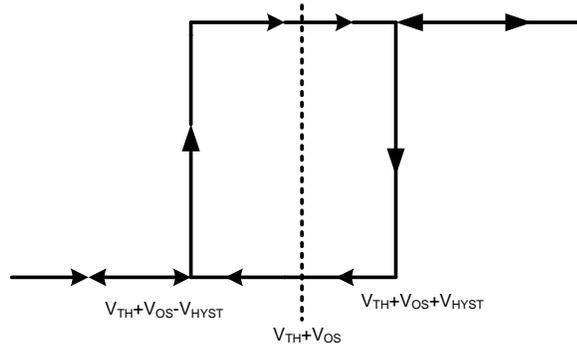
**Figure 15. AZV3001A Hysteresis Transfer Curve**
