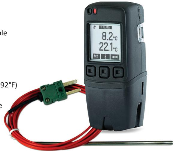
This standalone data logger measures and stores more than 250,000 temperature readings from two K, J or T-type thermocouple probes at a resolution of 0.1°C (0.2°F). It comes supplied with two K-type thermocouples capable of measuring from 0 to 200°C (32 to 392°F).
