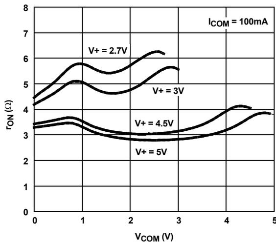
**FIGURE 10. ON-RESISTANCE vs SUPPLY VOLTAGE vs SWITCH VOLTAGE**
