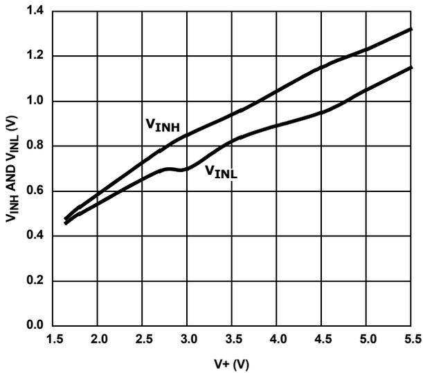
**FIGURE 16. DIGITAL SWITCHING POINT vs SUPPLY VOLTAGE**
