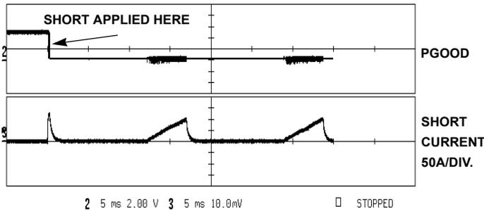
**FIGURE 6. SHORT APPLIED TO SUPPLY AFTER POWER-UP**
