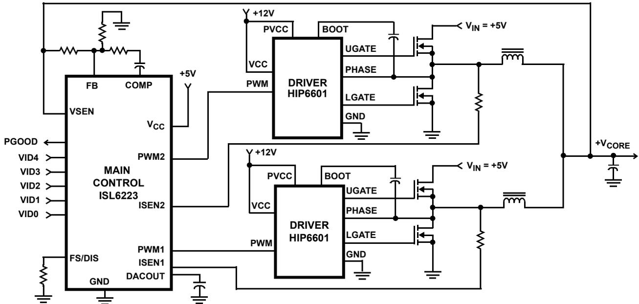
**Typical Application - Two Phase Converter Using a HIP6602 Gate Driver**
