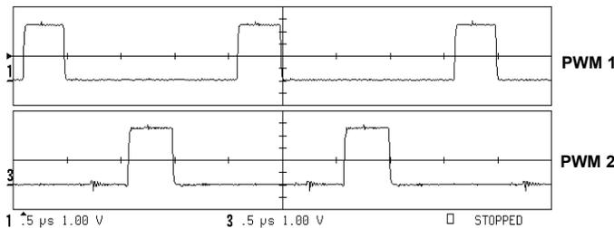
FIGURE 2. TWO PHASE PWM OUTPUT AT 500kHz
