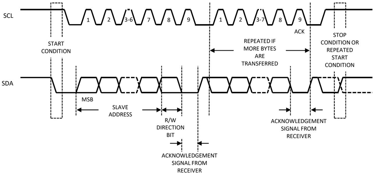
**Figure 7. Data Transfer on I<sup>2</sup>C Serial Bus**
