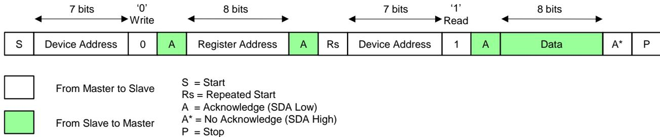
**Figure 9. I<sup>2</sup>C Read Cycle**
