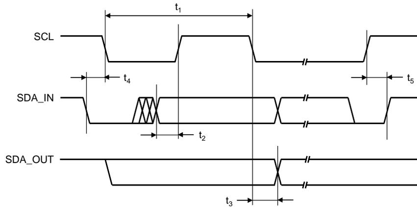
**Figure 1. I<sup>2</sup>C Compatible Interface Timing**
