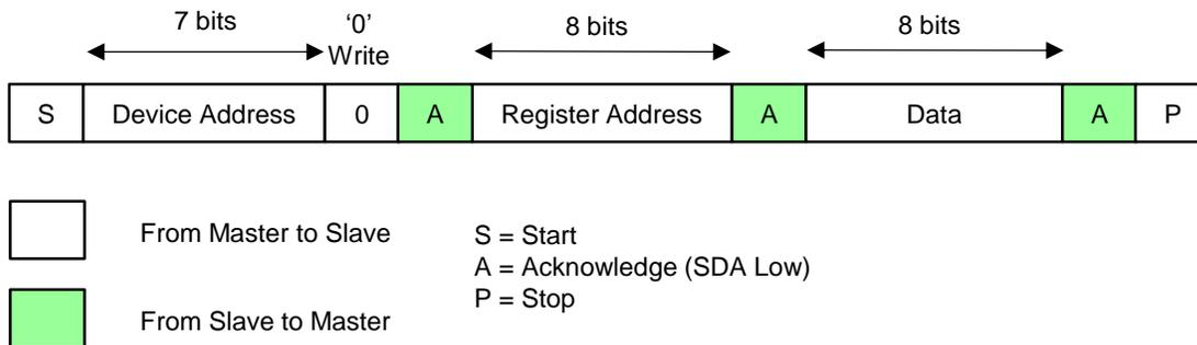
**Figure 8. I<sup>2</sup>C Write Cycle**
