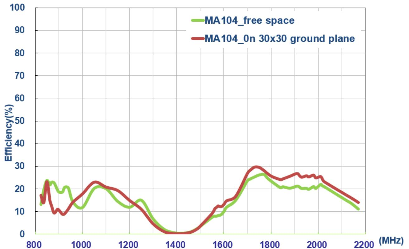
**Figure 8.** Efficiency of the MA104 antenna with 960~1700MHz
