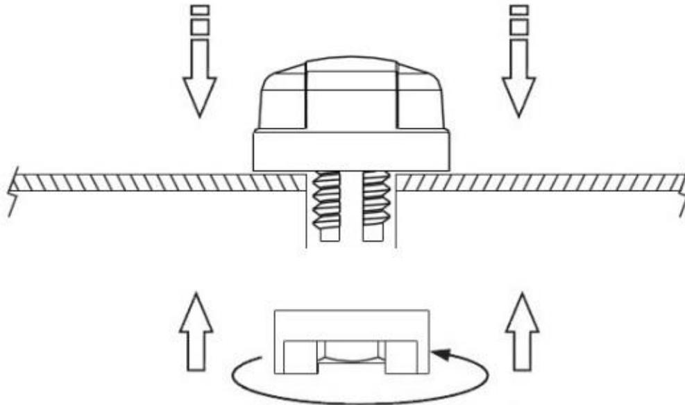
Recommended torque for Mounting is 24.5N·m
