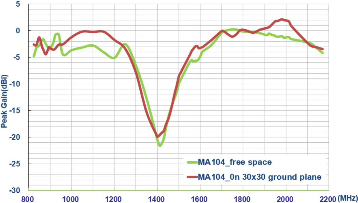
**Figure 12.** Gain of the MA104 antenna from 960~1700MHz
