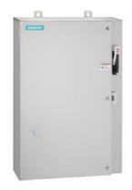
Non-reversing motor starter Size 1 Three phase full voltage Solid-state overload relay OLRelay amp range 5.5-22A 110VAC 50HZ / 120VAC 60HZ coil Combination type 30Amp fusible disconnect 30 Amp /600V fuse clip Encl NEMA type 4X 316 S-steel Water/dust tight non-corrosive Extra-wide enclosure
