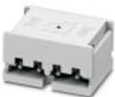
Plug component, Nominal current: 10 A, Rated voltage (III/2): 24 V, Number of positions: 4, Pitch: 2.4 mm, Color: white, Contact surface: Tin, Mounting: Direct plug-in method, for flexible PCBs with a width of 10 mm and a permissible PCB thickness in the contact zone of 0.15 mm ... 0.3 mm
