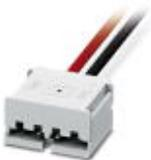
Plug component, Nominal current: 10 A, Rated voltage (III/2): 24 V, Number of positions: 2, Pitch: 2.4 mm, Color: white, Contact surface: Tin, Mounting: Direct plug-in method, Length of the punched-on cables: 500 mm, for flexible PCBs with a width of 10 mm and a permissible PCB thickness in the contact zone of 0.15 mm ... 0.3 mm
