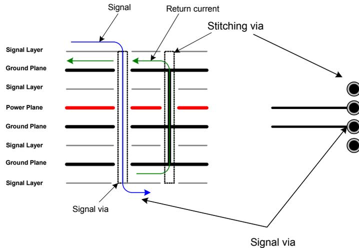
**Figure 2. Return current path utilizing stitching vias**
