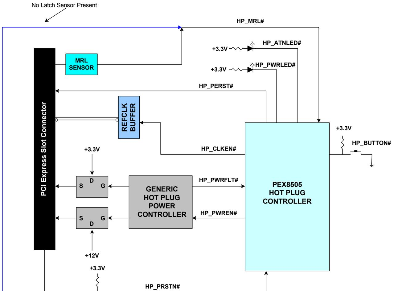
Figure 6. PEX 8505 Hot Plug Controller Interface
