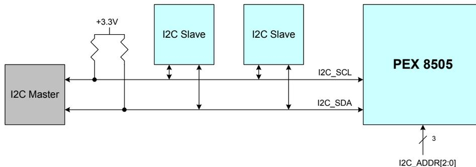
**Figure 5. I2C bus connectivity**
