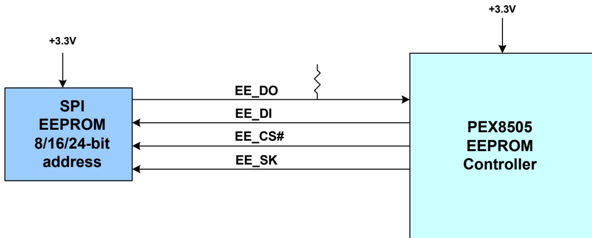
**Figure 4. PEX 8505 SPI EEPROM Interface**
