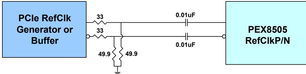
**Figure 3. PEX\_REFCLKP/N Implementation Example**
