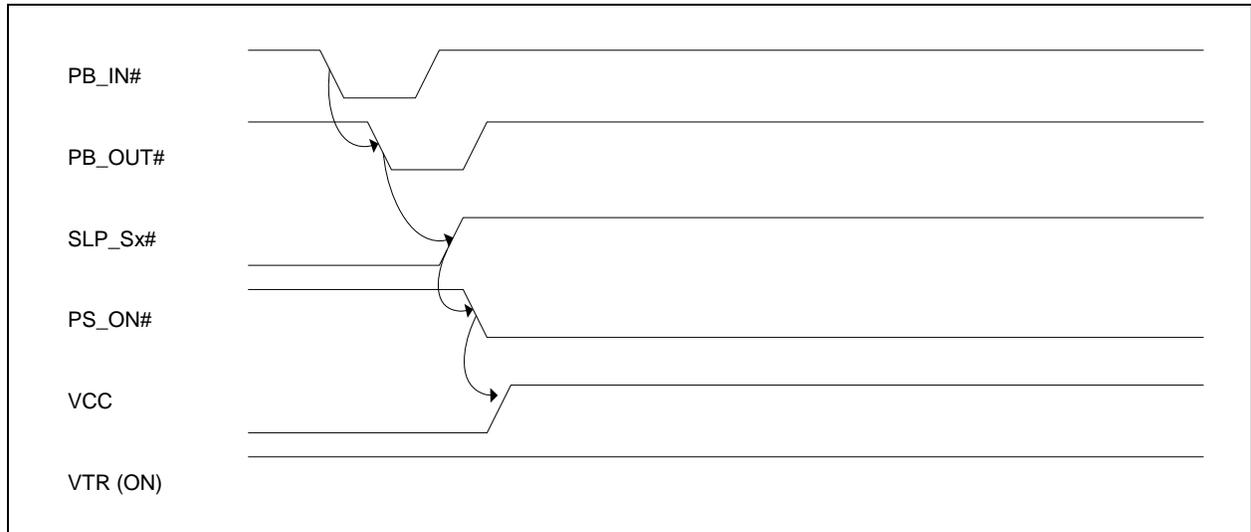
**FIGURE 18-4: POWER SUPPLY AFTER POWER FAILURE (RETURN TO OFF)**
