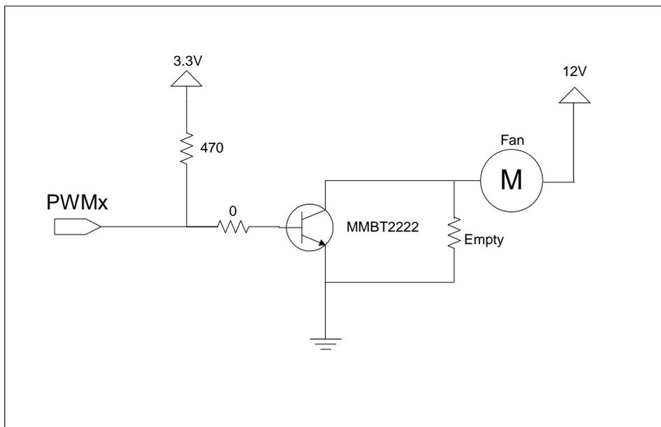
FIGURE B-3: FAN TACHOMETER CIRCUITRY (APPLY TO EACH FAN)
