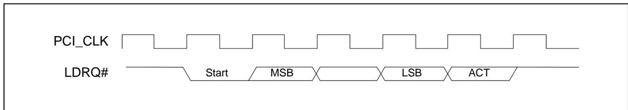
**FIGURE 27-10: DMA WRITE (FIRST BYTE)**
