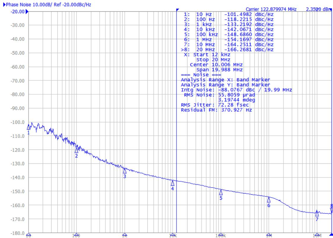
Figure 8.1.  $f_{IN} = 156.25\text{ MHz}$ ,  $f_{OUT} = 122.88\text{ MHz}$
