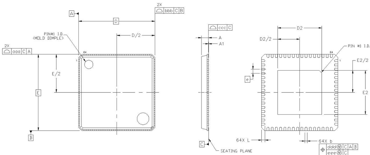
Figure 10.1. Si5386 9x9 mm 64-QFN Package Diagram
