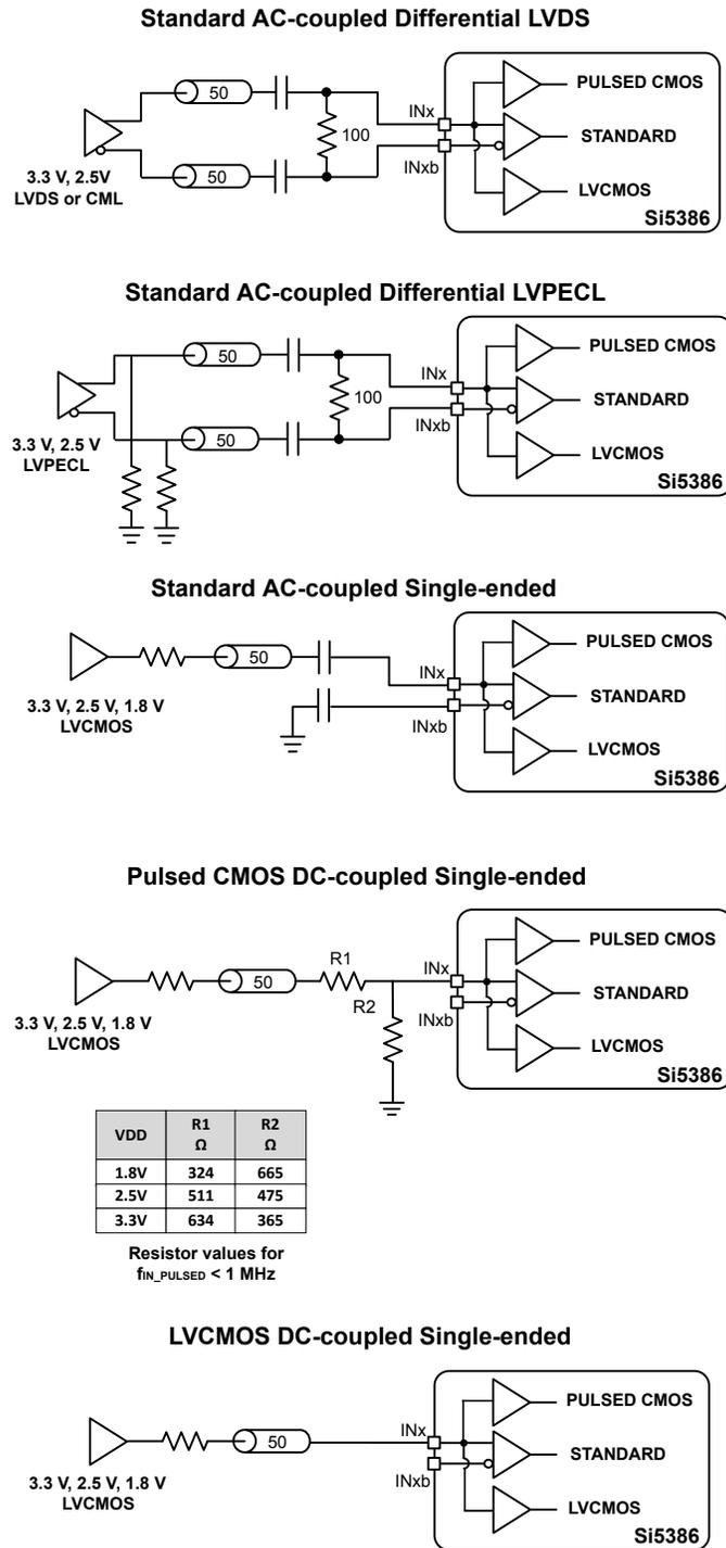
Figure 3.4. Termination of Differential and LVCMOS Input Signals
