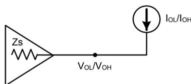
**AC Output Test Configuration**
