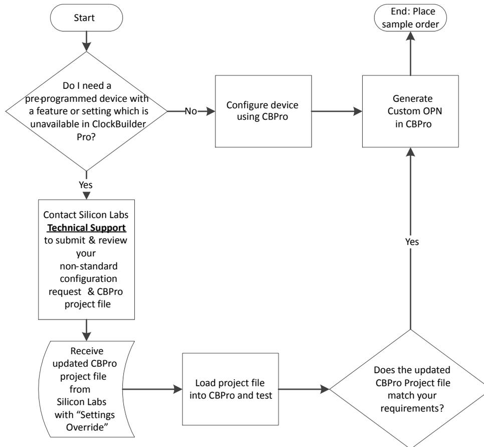
**Figure 3.14. Process for Requesting Non-Standard CBPro Features**
