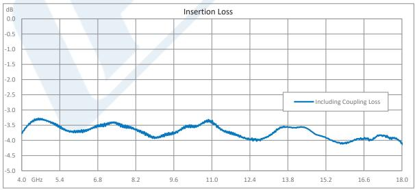
Click the following link (or enter part number in "SEARCH" on website) to obtain additional part information including price, inventory and certifications: 180 Degree SMA Hybrid Coupler from 4 GHz to 18 GHz Rated to 50 Watts PE2CP1160
