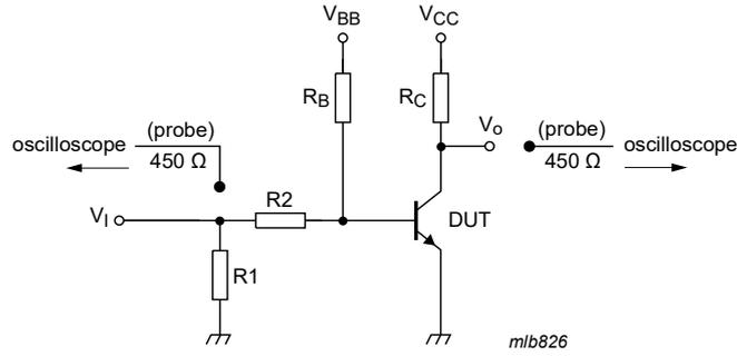
Fig. 7. Test circuit for switching times
