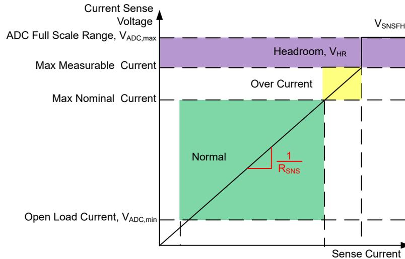
Figure 8-2. Voltage Indication on the Current-Sense Pin
