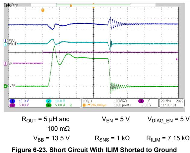
Figure 6-23. Short Circuit With ILIM Shorted to Ground
