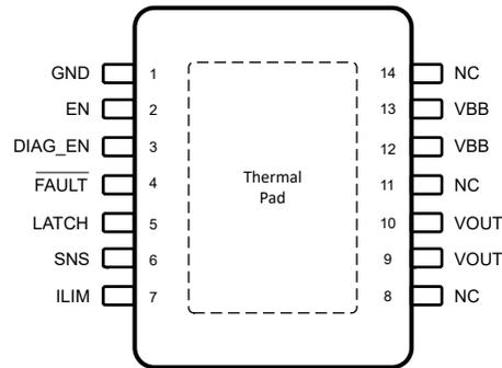
**Figure 5-1. PWP Package, 14-Pin HTSSOP (Top View)**
