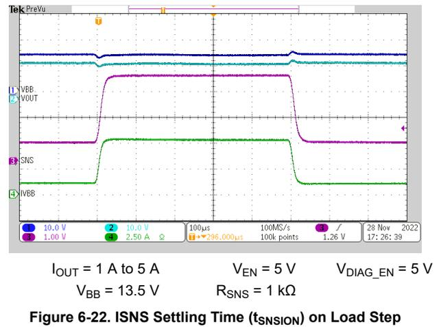
Figure 6-22. ISNS Settling Time ( $t_{SNSION}$ ) on Load Step
