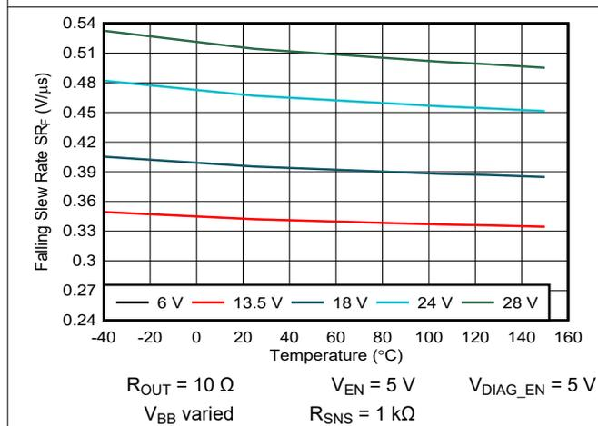
Figure 6-17. Falling Slew Rate SRF vs Temperature
