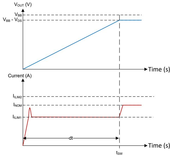
**Figure 9-4. Large Capacitive Charging Changing Current Limit**
