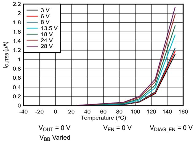
Figure 6-3. Output Leakage Current  $I_{OUT,STBY}$  vs Temperature
