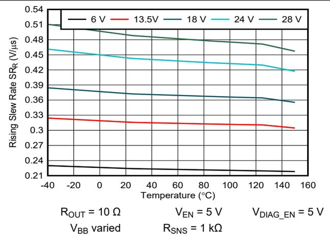
Figure 6-16. Rising Slew Rate SRR vs Temperature
