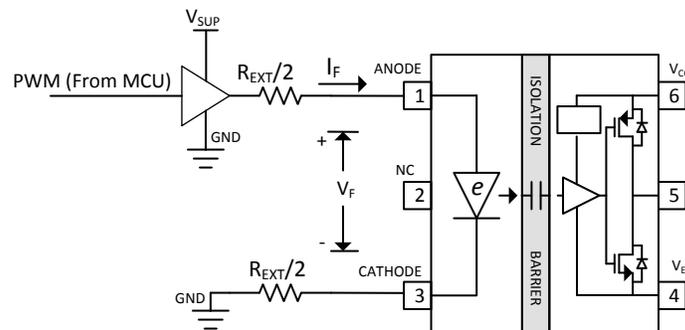
$$R_{EXT} = \frac{V_{SUP} - V_F}{I_F} - R_{OH\_buf}$$
