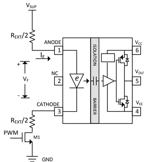
$$R_{EXT} = \frac{V_{SUP} - V_F}{I_F} - R_{M1}$$
