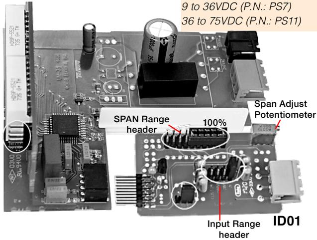
Decimal selection is made by moving the jumper to the indicated position on the header for the decimal required on the front of the display board.
