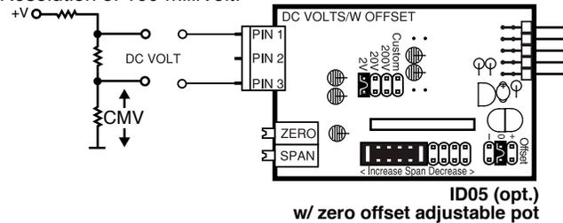
Max CMV (common mode voltage) is 50V.\*
