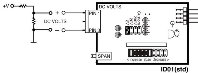
**DC Volts Differential** measurement with a Resolution of 100 milliVolt.
