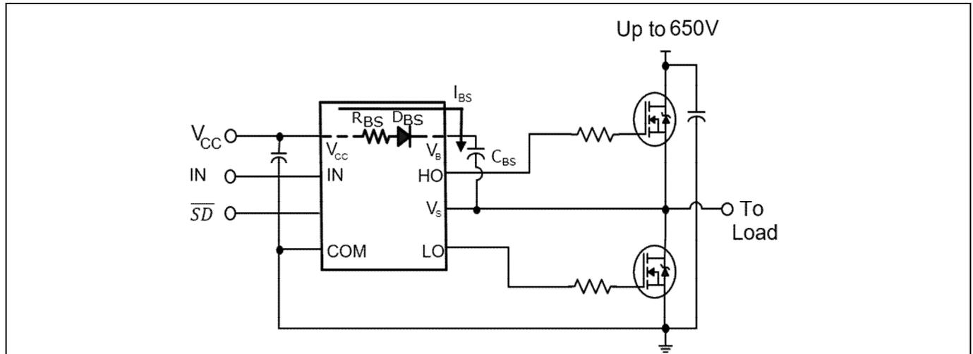
**Figure 17** Half bridge bootstrap circuit in 2ED218x
