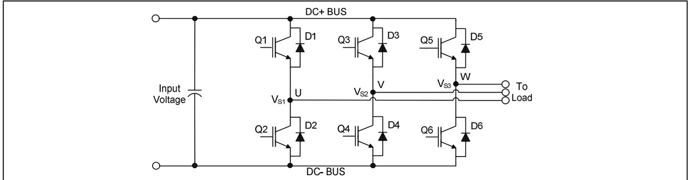
Figure 19 Three phase inverter
