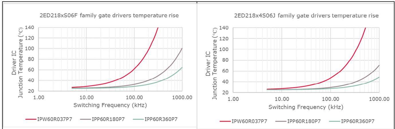
\*Assumptions for above curves:  $T_a = 25\text{ }^\circ\text{C}$ ,  $V_{BUS} = 400\text{ V}$ ,  $V_{CC} = 12\text{ V}$ ,  $R_{gon} = 10\ \Omega$ ,  $R_{goff} = 5\ \Omega$
