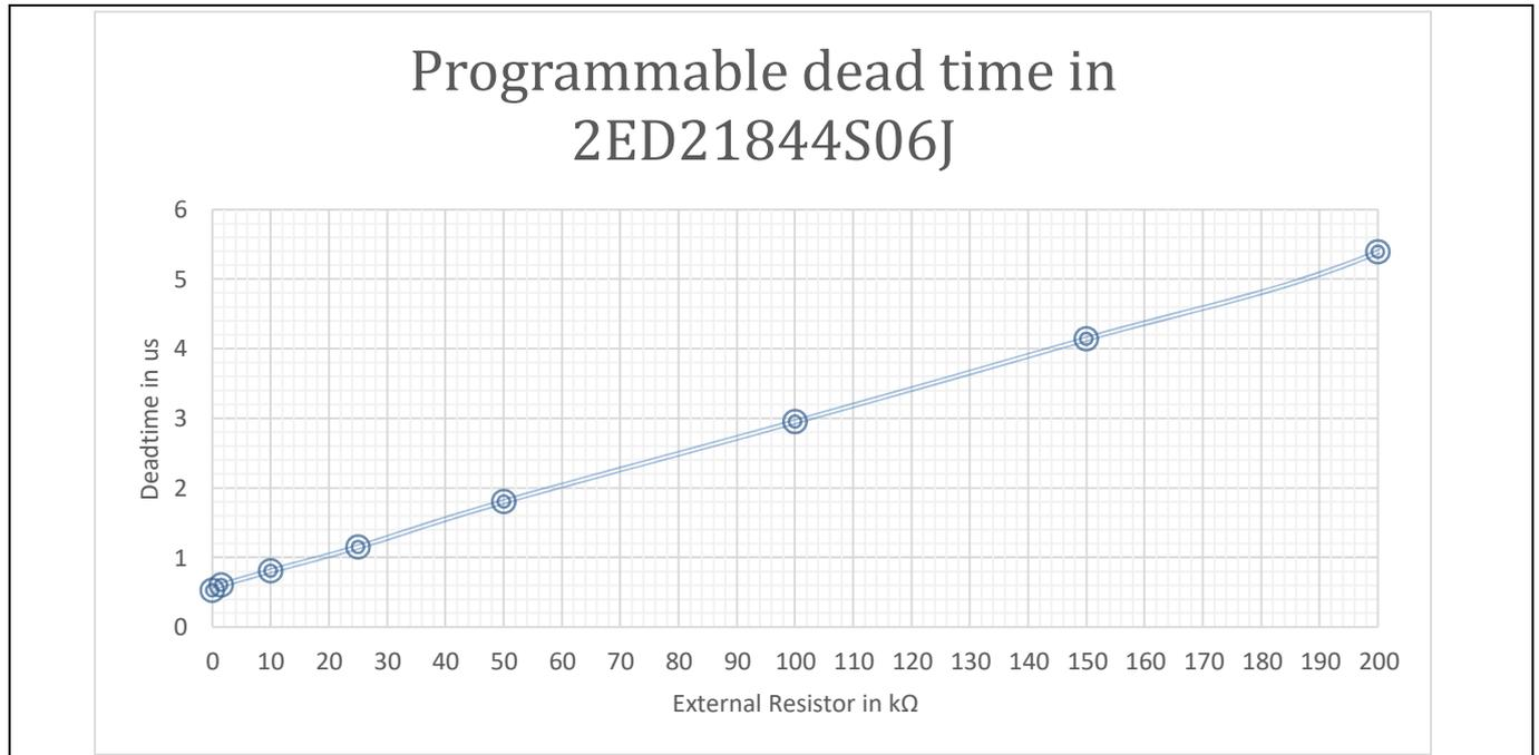
Figure 11 Variation of dead time vs. external resistor
