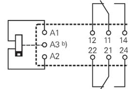
a) Indicated contact position while or after coil energization with reset voltage.
