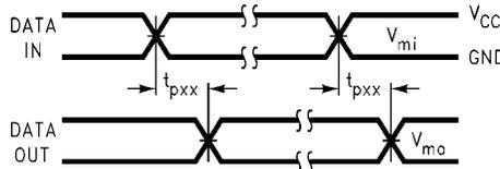
**FIGURE 6. Waveform for Inverting and Non-Inverting Functions**
