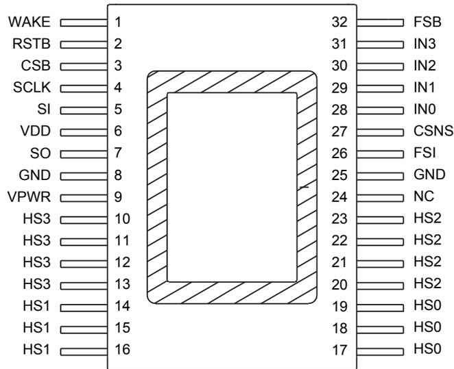
Figure 3. 10XS3425 pin connections
