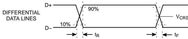
**Figure 4. USB Line Rise and Fall Times**
