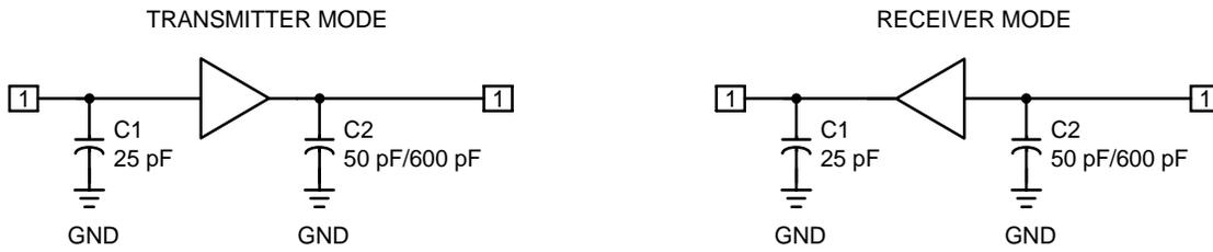
Figure 7. Input/Output Stray Capacitance Definitions
