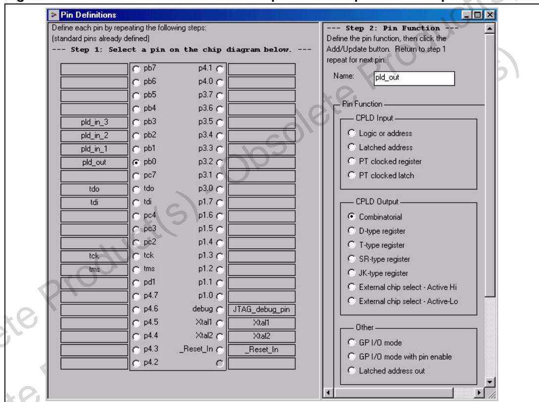
Figure 82. Using the design assistant in PSDsoft Express for simple PLD example
