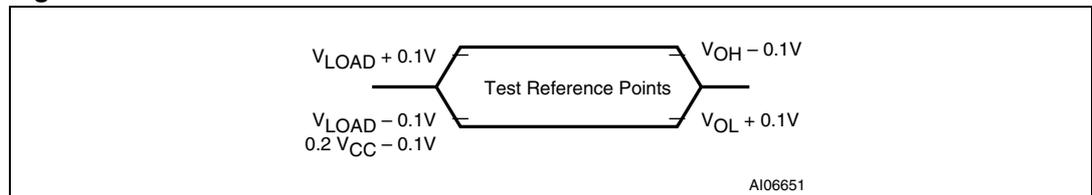
1. For timing purposes, a port pin is considered to be no longer floating when a 100 mV change from load voltage occurs, and begins to float when a 100 mV change from the loaded  $V_{OH}$  or  $V_{OL}$  level occurs
