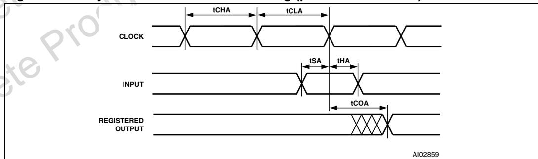
**Table 224. CPLD macrocell asynchronous clock mode timing (5 V PSD module)**
