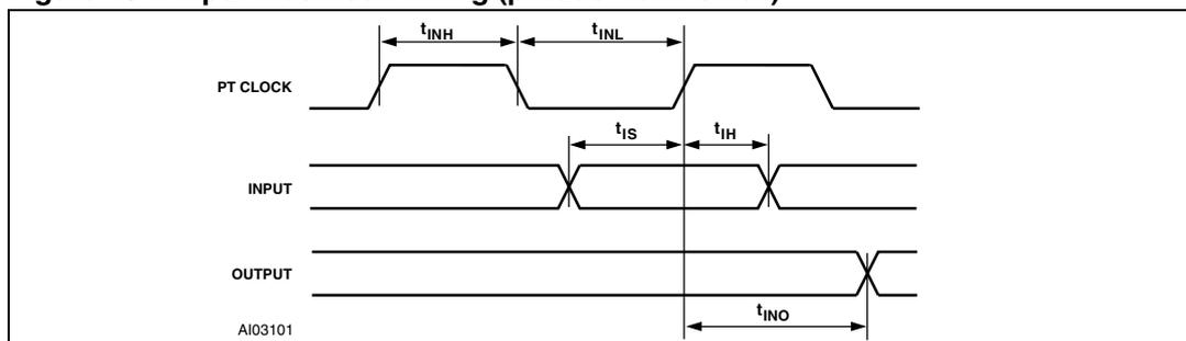
Table 226. Input macrocell timing (5 V PSD module)
