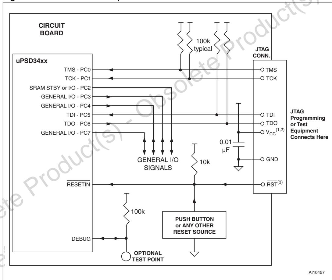
1. For 5 V UPSD34xx devices, pull-up resistors and  $V_{CC}$  pin on the JTAG connector should be connected to 5 V system  $V_{DD}$ .
