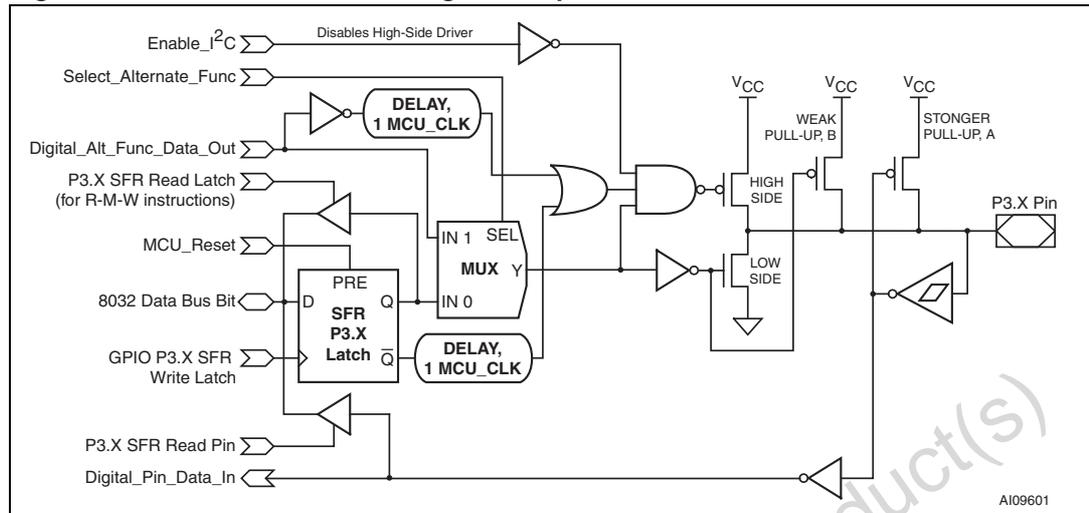
Figure 18. MCU I/O cell block diagram for port 4
