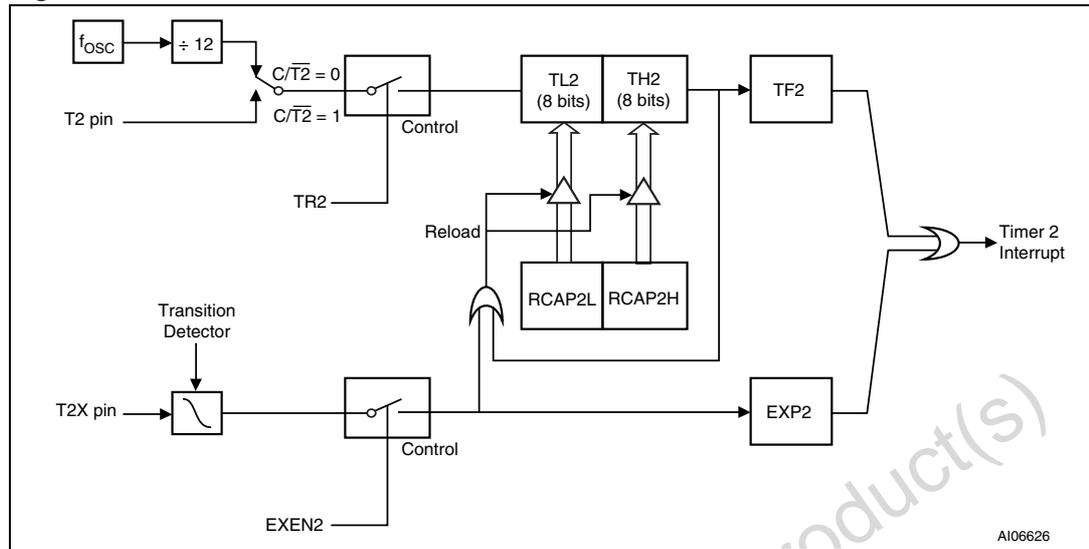
Figure 29. Timer 2 in baud rate generator mode
