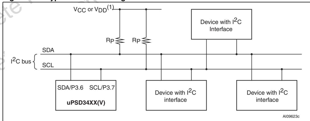
1. For 3.3 V system, connect R<sub>P</sub> to 3.3 V V<sub>CC</sub>. For 5.0 V system, connect R<sub>P</sub> to 5.0 V V<sub>DD</sub>.
