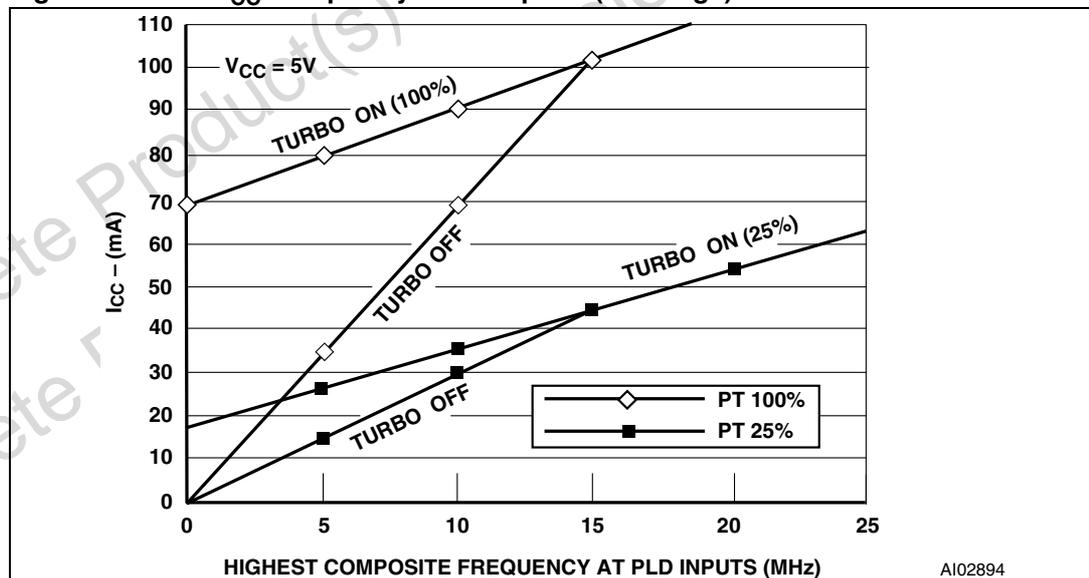
Figure 96. PLD I<sub>CC</sub> / frequency consumption (3 V range)
