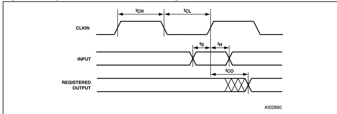
Table 222. CPLD macrocell synchronous clock mode timing (5 V PSD module)
