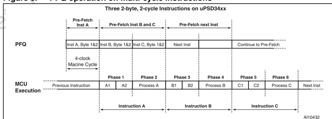
Figure 9. UPSD34xx multi-cycle instructions compared to standard 8032
