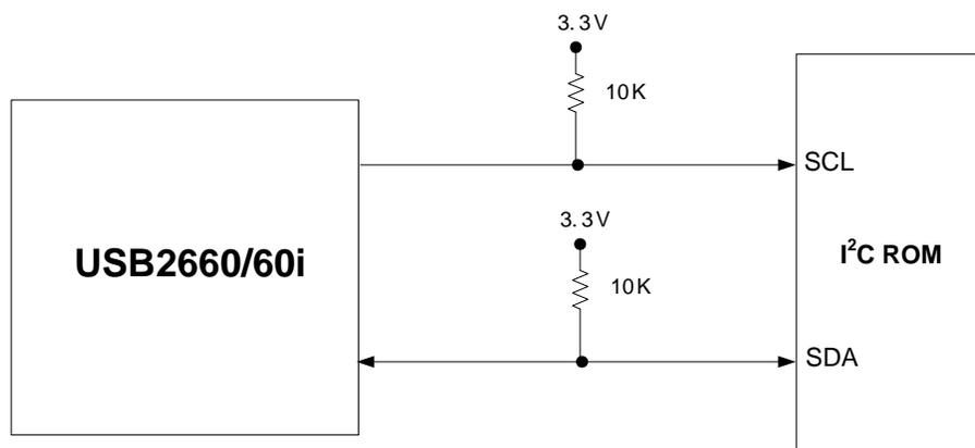
Figure 6.5 I<sup>2</sup>C Connection
