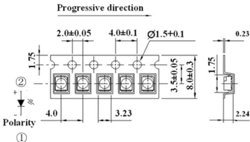
Note: Tolerances unless mentioned  $\pm 0.1$ mm. Unit = mm
