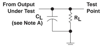
NOTE A:  $C_L$  includes probe and jig capacitance.
