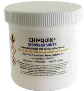
**\*Shelf Life Notes:** Chip Quik® solder paste is good past its quoted shelf life, regardless of refrigeration. Before use, visually inspect the solder paste to ensure it is not dried out or clumpy, or check stencil release. If stored in a jar, stir the product thoroughly for 2-3 minutes before inspection and use.
